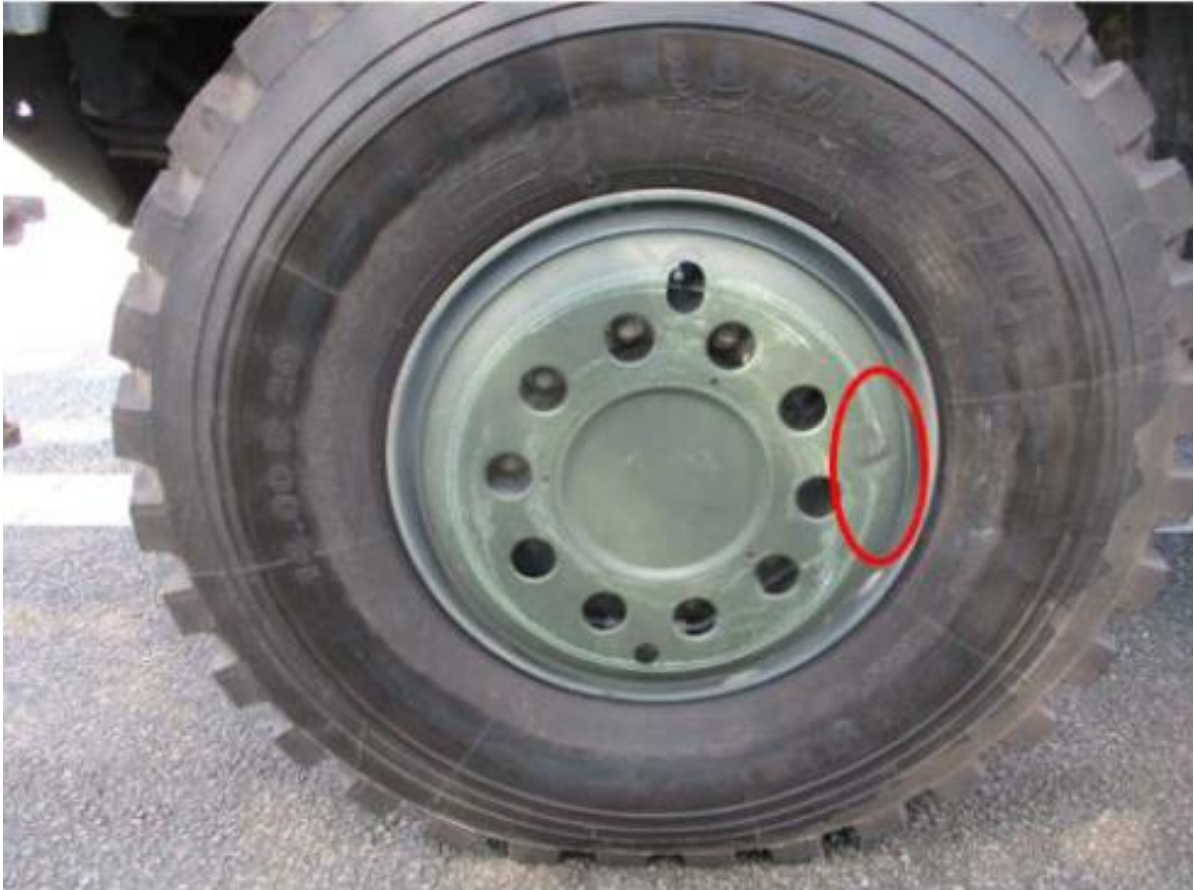
Figure B-5: Close-up View of Damaged Area of MID20364 Damage Assessment: MID20364 left-front rim cover sustained scratches and dents
