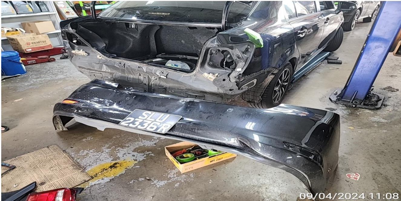
REAR BUMPER DEFORMED
