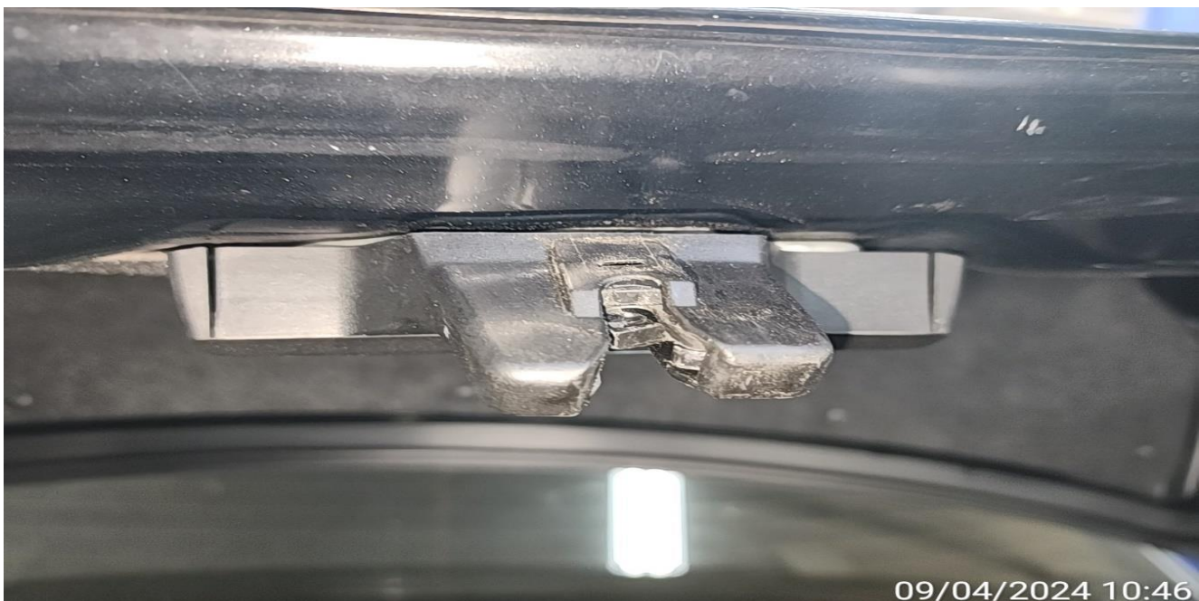
BOOTLID LOCK DISTORTED
