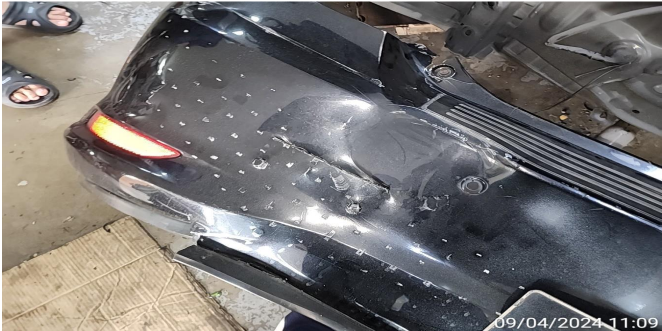
REAR REVERSE SENSOR DISTORTED
