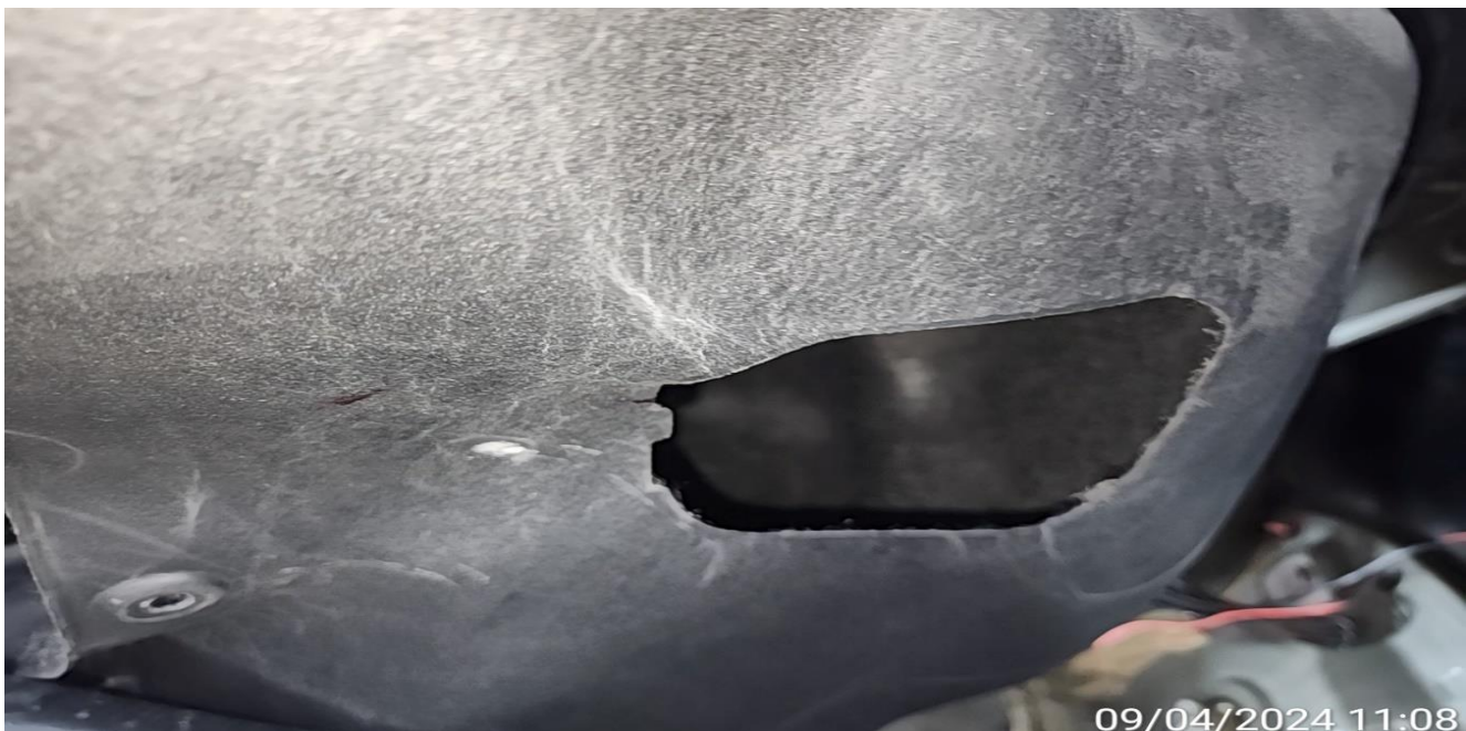
REAR FENDER INNER TRIM CRACKED
