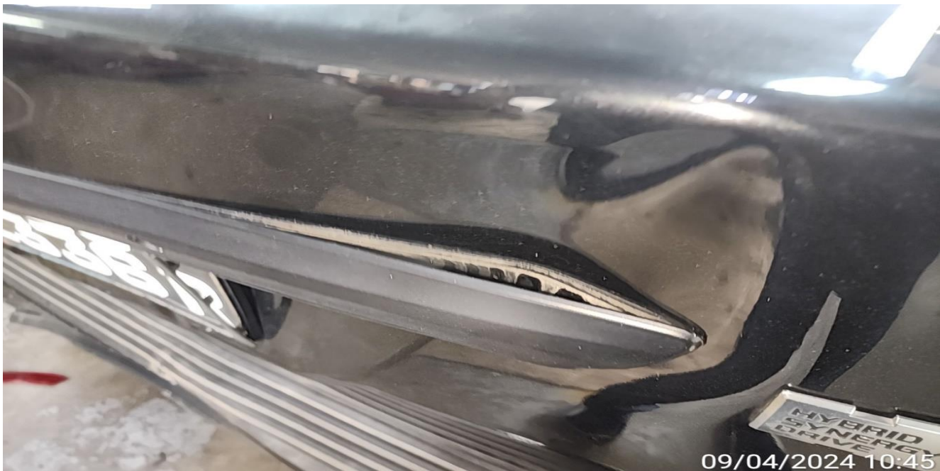
BOOTLID OUTER CHROME GARNISH CRACKED
