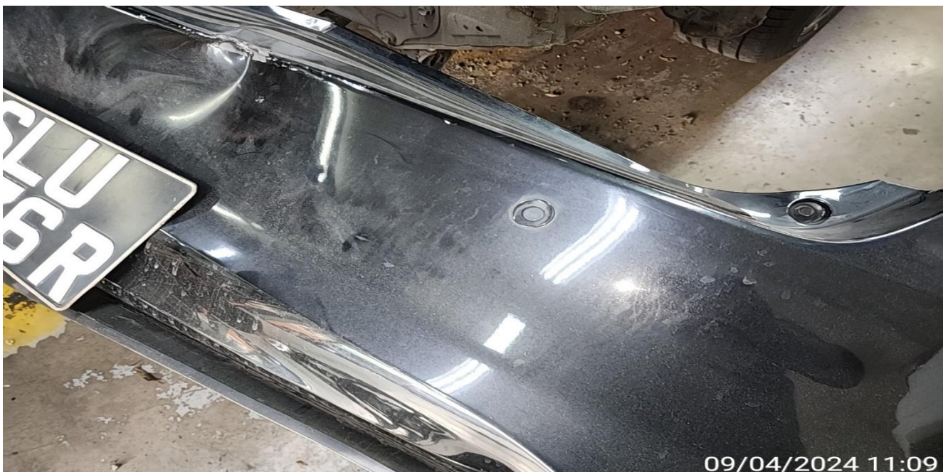
REAR REVERSE SENSOR DISTORTED
