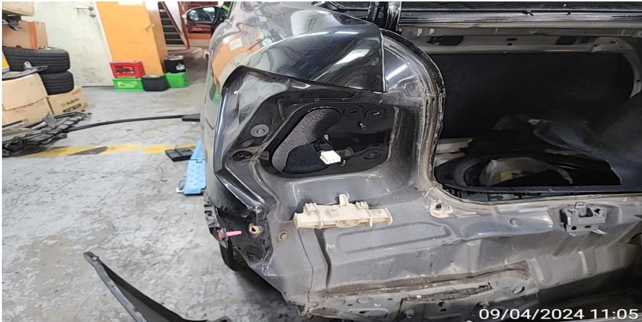
TAILLAMP PANEL LH BUCKLED
