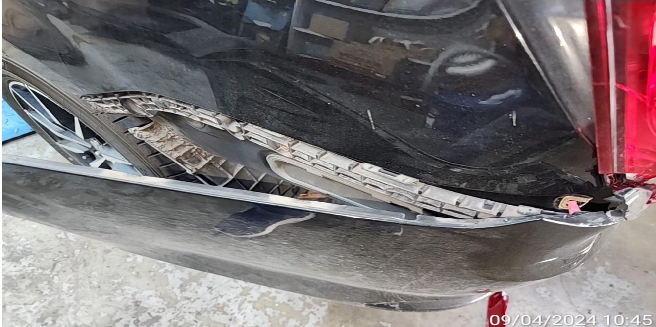
REAR BUMPER SIDE RETAINER CRACKED
