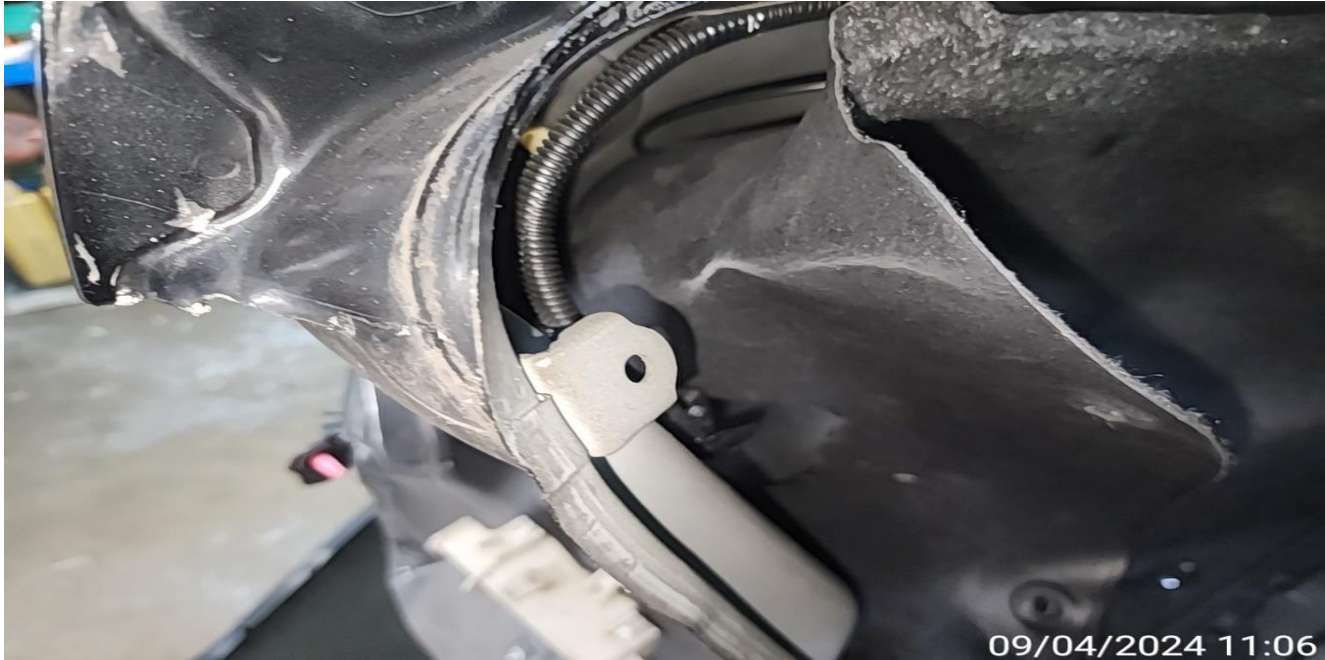
REAR FENDER INNER TRIM CRACKED
