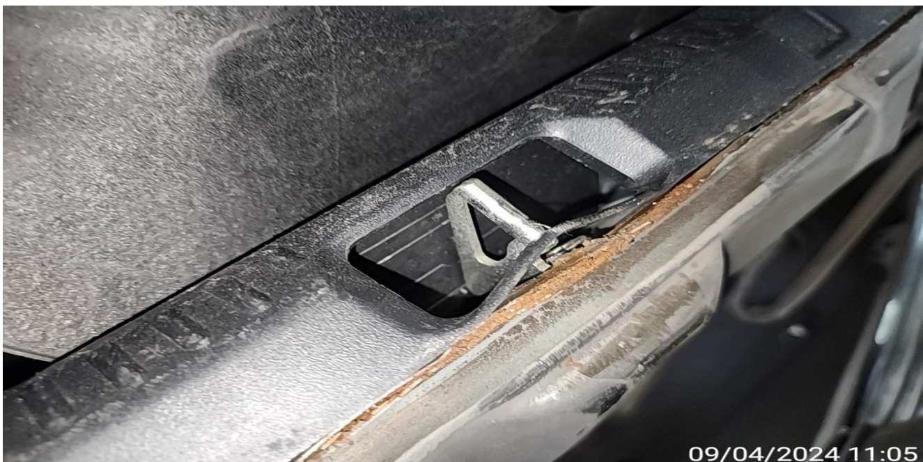
REAR END PANEL INNER TRIM DEFORMED
