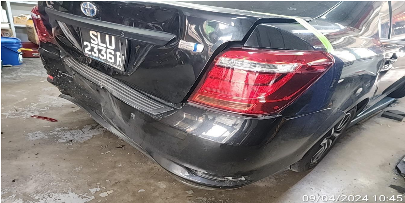
REAR BUMPER DEFORMED
