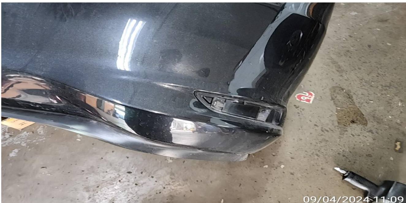
REAR BUMPER REFLECTOR CRACKED/ MISSING
