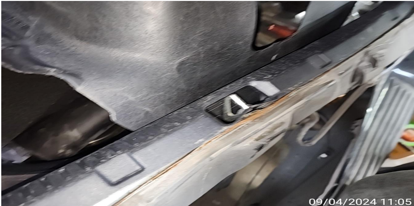
REAR END PANEL INNER TRIM DEFORMED
