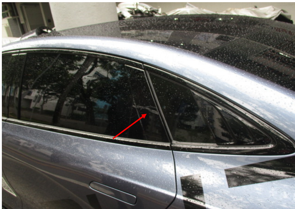
Photo 5 shows upon closer examination of the left rear door, we observed horizontal graze marks on the left rear door trim of the BYD (arrowed).
