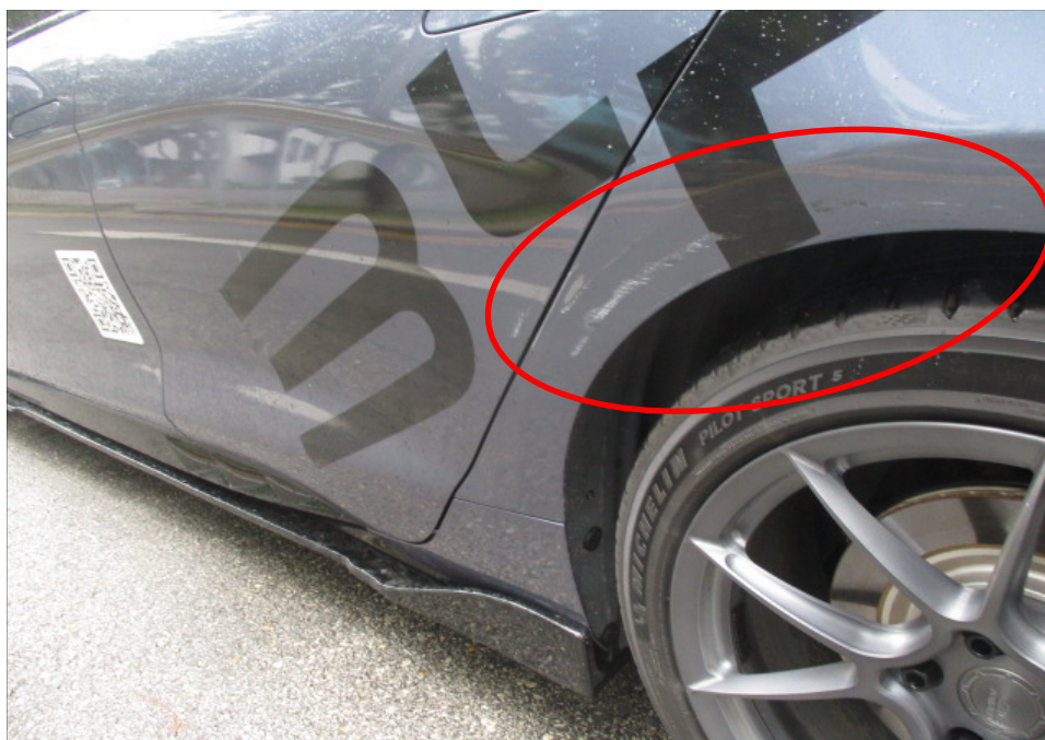
Photo 3 shows upon closer examination of the left rear portion, we observed horizontal paint graze marks on the left rear fender of the BYD (circled).
