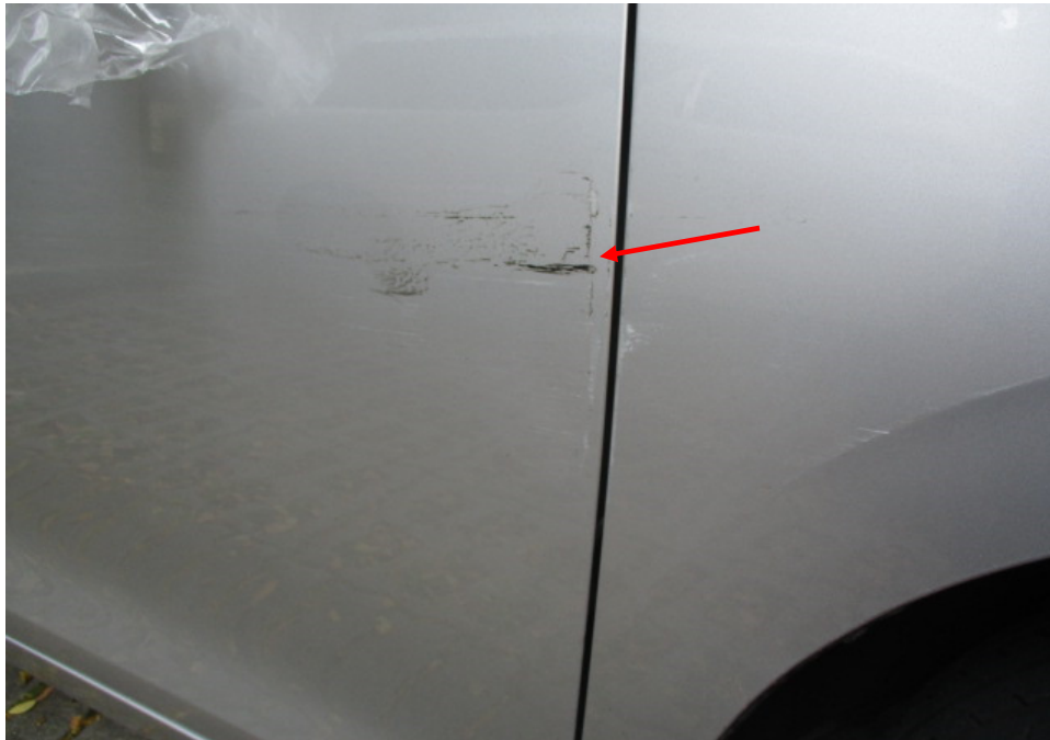
Photo 11 shows a close up view of the horizontal paint graze marks on the right front door of the Toyota (arrowed).
