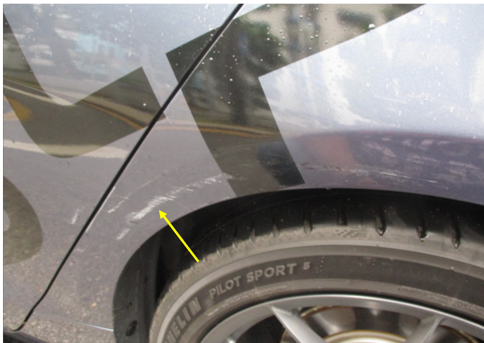
Photo 4 shows a close up view of the horizontal paint graze marks on the left rear fender of the BYD (arrowed).
