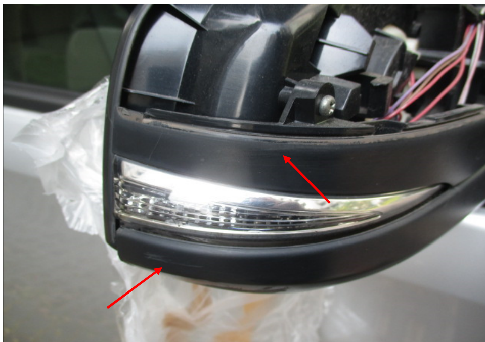
Photo 13 shows upon closer examination of the right side mirror, we observed horizontal graze marks (arrowed).
