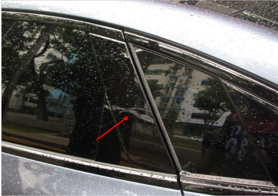
Photo 6 shows a closer view of the horizontal graze marks on the left rear door trim of the BYD (arrowed).
