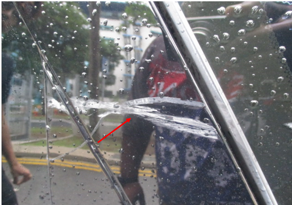
Photo 7 shows a close up view of the horizontal graze marks on the left rear door trim of the BYD (arrowed).
