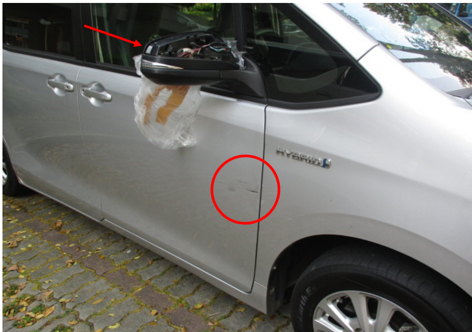
Photo 10 shows upon closer examination of the right frontal portion, we observed horizontal paint graze marks on the right front door (circled) and the deformed right side mirror (arrowed) of the Toyota.
