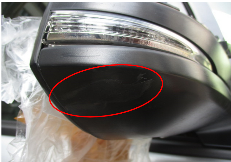
Photo 14 shows more horizontal graze marks on the underside of the right side mirror of the Toyota (circled).
