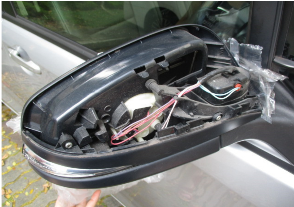
Photo 12 shows the right side mirror of the Toyota with its cover missing.
