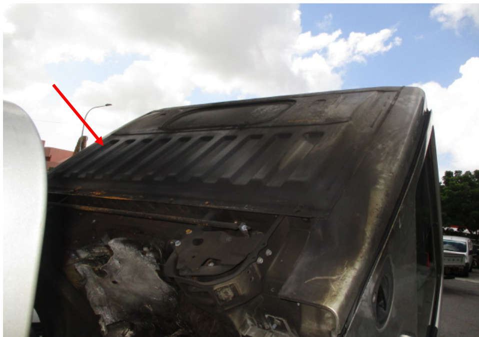
Photo 5 shows the cab of the Insured Vehicle at the time of our inspection. The damage to the cab of the Insured Vehicle was confined to its rear portion (arrowed).
