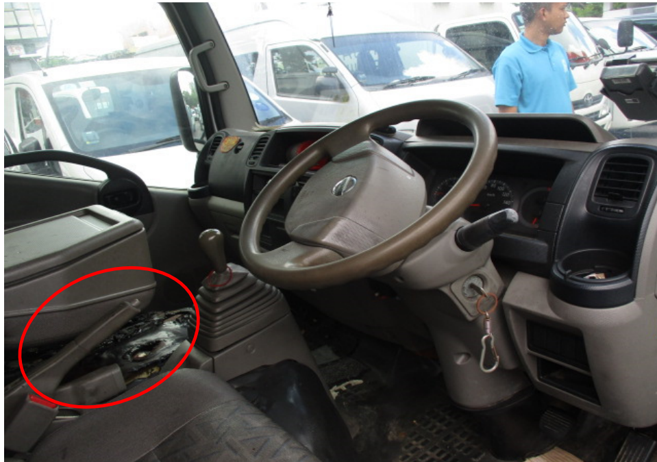
Photo 3 shows the interior compartment the Insured Vehicle at the time of our inspection. The centre portion of the interior compartment of the Insured Vehicle was severely affected by the fire (circled).
