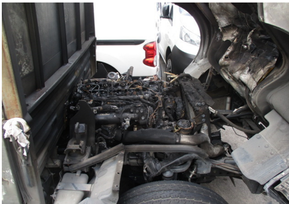
Photo 6 shows the engine compartment of the Insured Vehicle which is situated beneath the cab at the time of our inspection. The engine compartment of the Insured Vehicle was seriously affected by the fire.
