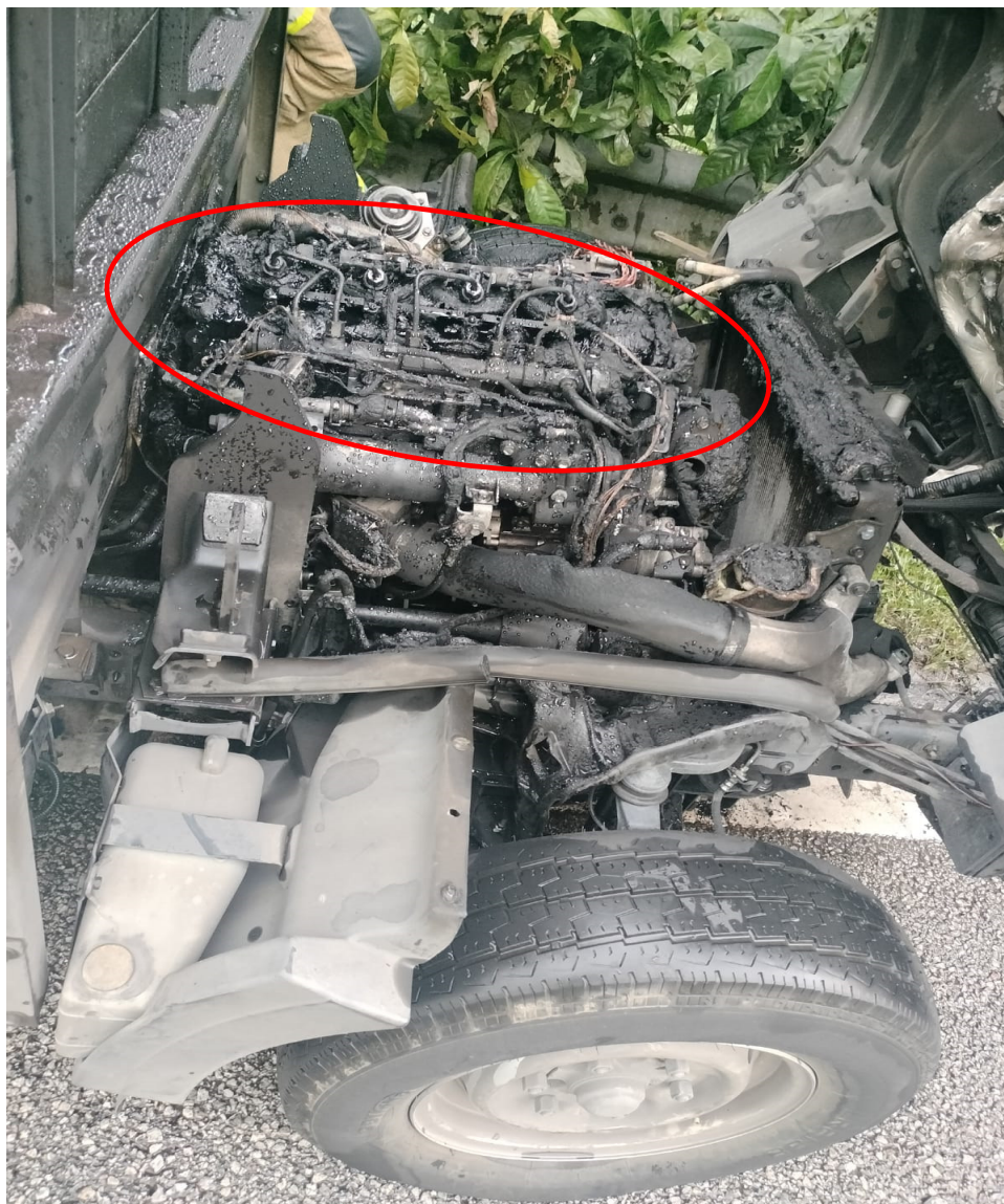
Photo 15 shows the engine compartment of the Insured Vehicle after firefighters were able to lift the cab post- incident. In general, the damages sustained to the engine compartment and the fire extinguisher water residue found on the burnt stretches of wirings (circled) had corresponded to the events that were related to us by Mr Gazi, which is the fire had started from the engine compartment.
