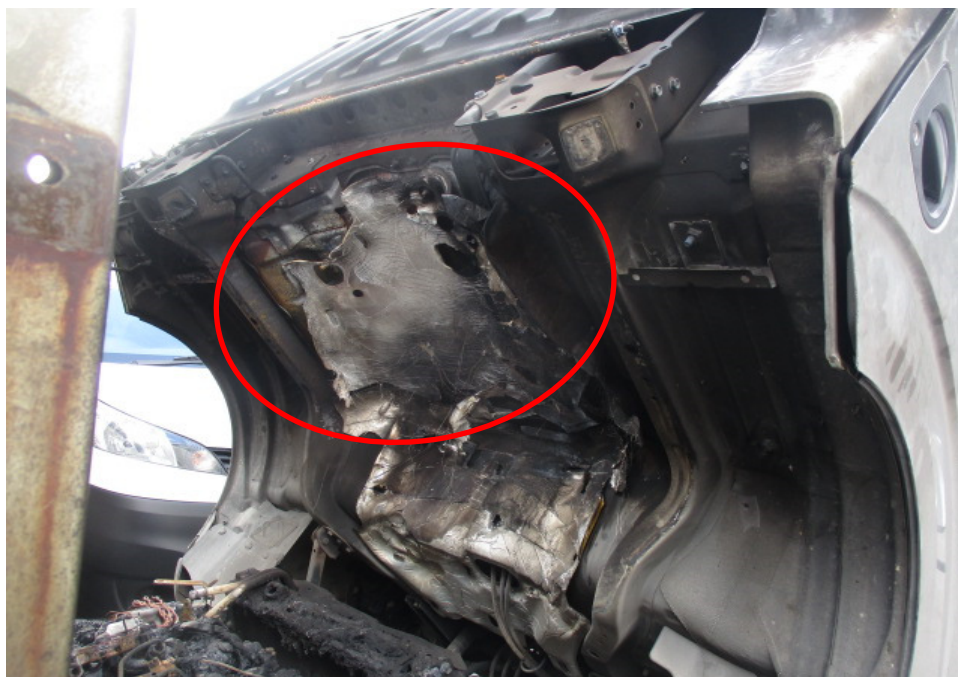
Photo 7 shows the whitish burn marks that were found on the underside of the cab of the Insured Vehicle (circled). Such whitish burn marks are a result of exposure to prolonged heat intensity.
