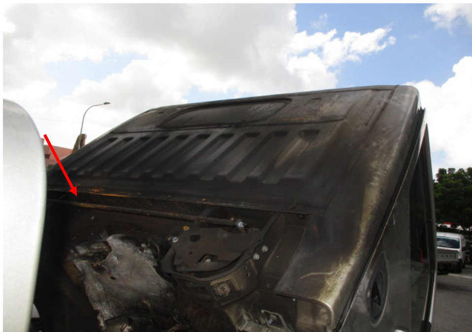
Photo 8 shows the rust that had developed on the cab mounting bracket of the Insured Vehicle (arrowed) which is an indication that the fire to the Insured Vehicle had originated from the engine compartment. The development of rust is an indication that the area was exposed to prolonged exposure to high heat intensity, which had caused the steel/metal material of the passenger side engine access panel to be exposed to natural environmental condition.
