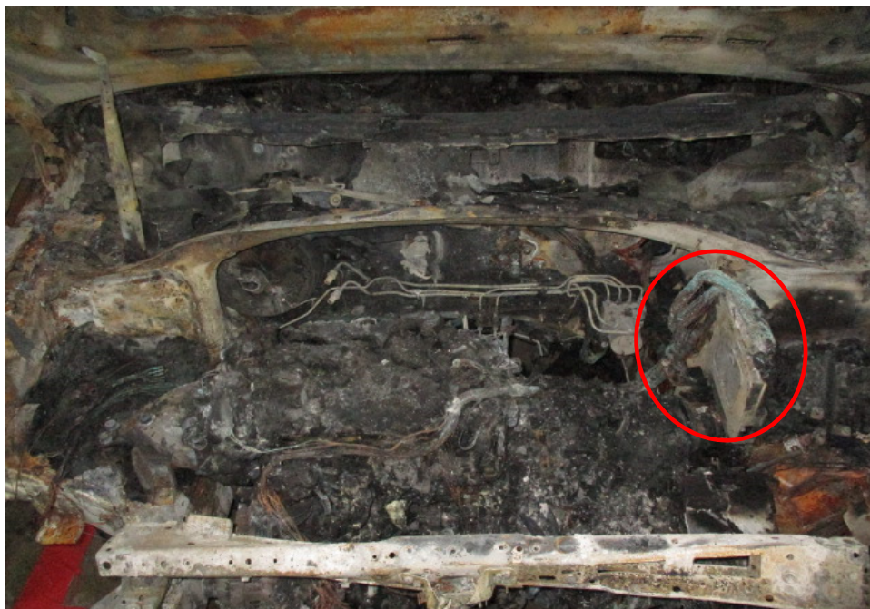
Photo 7 shows the wirings around the left rear portion of the engine compartment, which is in the immediate vicinity where the fire to the Insured Vehicle had likely started. We noticed greenish residue on several stretches of burnt wirings (circled). The presence of greenish residue indicates internal heating of copper wires, a sign of an electrical short circuit occurring.
