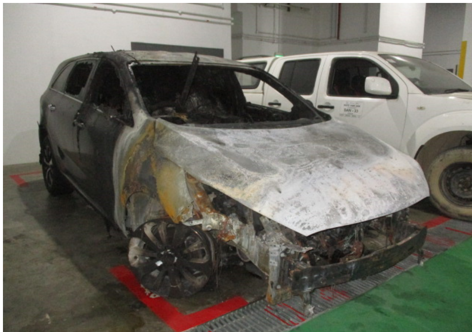
Photo 3 shows the closer view of the right front body of the Insured Vehicle at the time of our inspection. The fire damage to the Insured Vehicle was confined to its frontal portion. Its front bumper, front bonnet, headlamps, front windscreen, front wheel rims, front fenders and front tyres were amongst the body parts that were found to have been affected by the fire.
