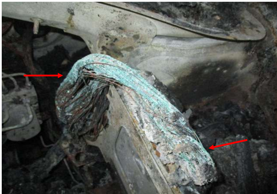
Photo 9 shows a close up view of the greenish residue found on several stretches of burnt wirings leading from the ECM of the Insured Vehicle (red arrows). The presence of such greenish residue suggests occurrence of an electrical short circuit.
