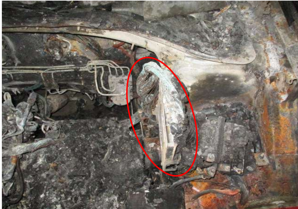
Photo 8 shows a closer view of the burnt wirings around the left rear portion of the engine compartment. We noticed greenish residue on several stretches of the burnt wirings leading from the Engine Control Module (ECM) (circled). The greenish residue is normally left behind from oxidation as a result of chemical reaction involving the copper wires.
