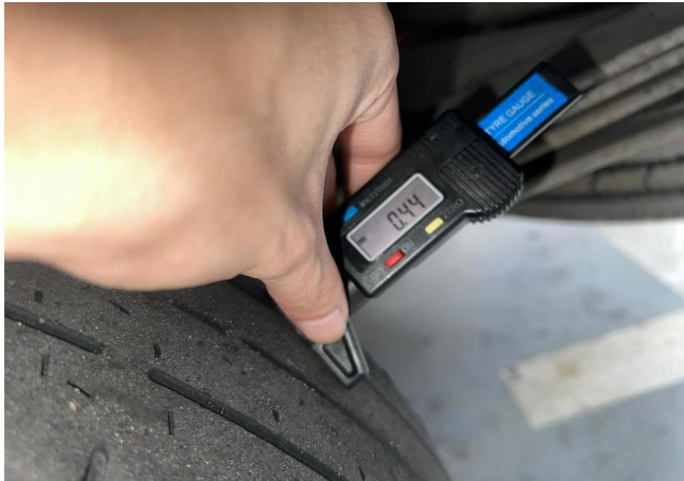
Photo 17 shows the tread depth of the rear left inner tyre (inner tread) on the insured vehicle at the time of my inspection. The remaining tread depth is 0.4mm which is not within the LTA requirements.
