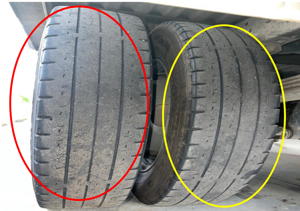
Photo 18 shows the general view of the rear left tyre tyres of the insured vehicle at the time of my inspection. The rear left tyres of the insured vehicle with remaining tread depth of 0.3mm- 0.9mm on the rear left outer tyre (red circle) and 0.4mm- 0.9mm on the rear left inner tyre (yellow circle).
