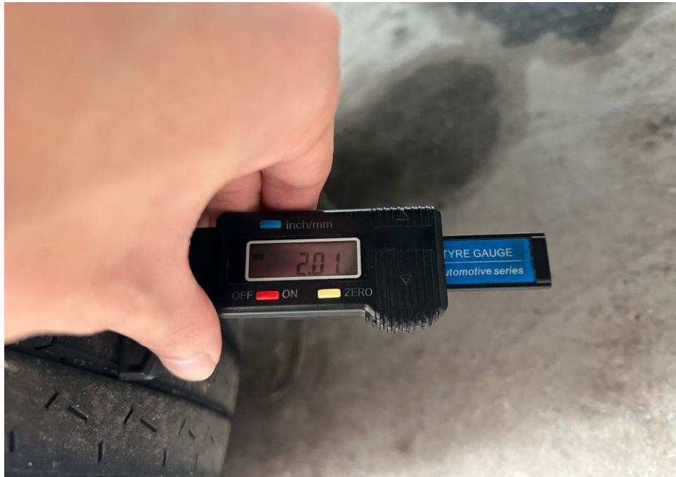
Photo 9 shows the tread depth of the rear right outer tyre on the insured vehicle at the time of my inspection. The remaining tread depth is 2.0mm which is within the LTA requirements.
