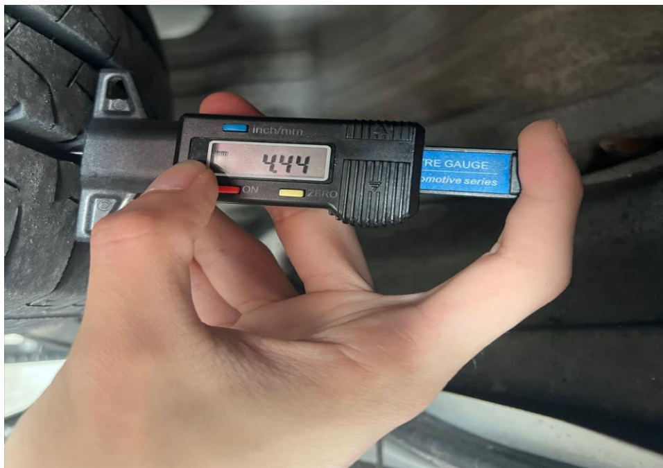
Photo 5 shows the tread depth of the front right tyre on the insured vehicle at the time of my inspection. The remaining tread depth is 4.4mm which is within the LTA requirements.
