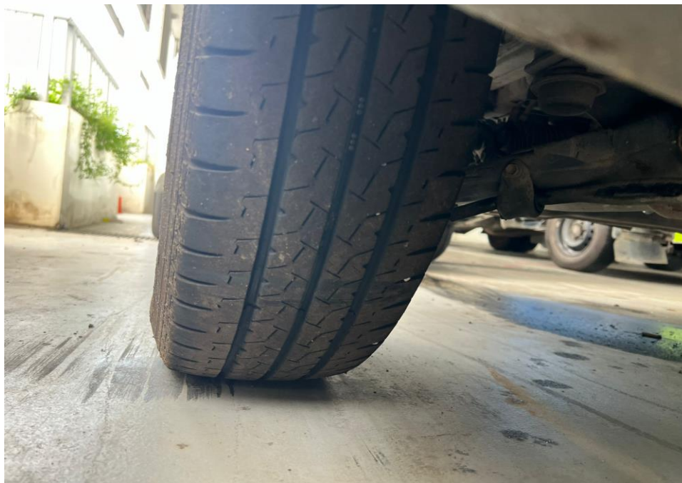
Photo 8 shows the front left tyre of the insured vehicle at the time of my inspection. The front left tyre of the insured vehicle was observed to be in serviceable condition with the remaining tread depth of 4.8mm which is within LTA requirements.
