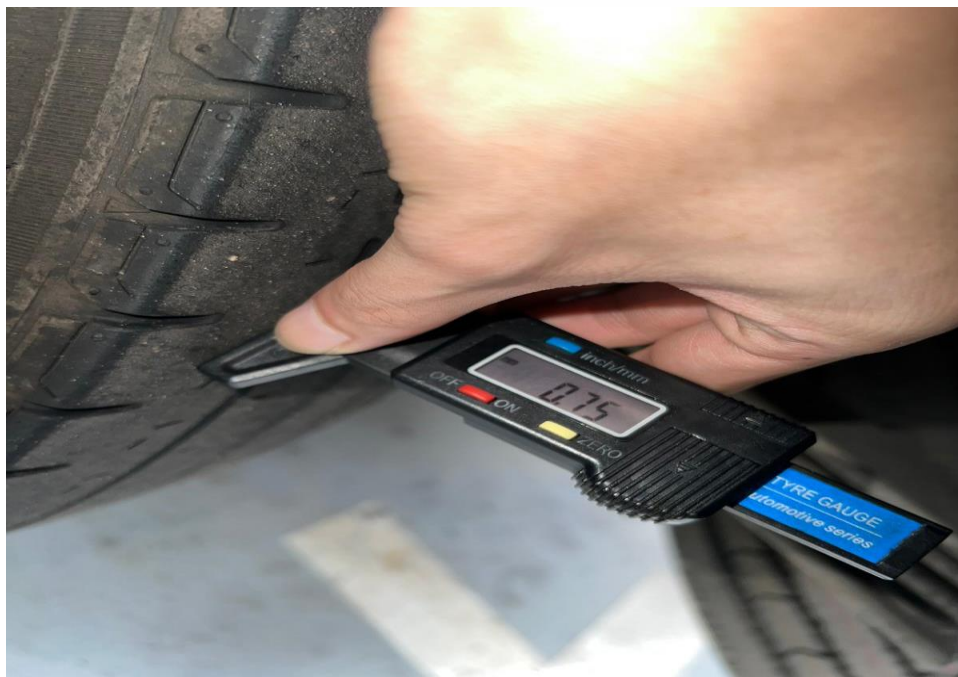
Photo 15 shows the tread depth of the rear left inner tyre (outer tread) on the insured vehicle at the time of my inspection. The remaining tread depth is 0.7mm which is not within the LTA requirements.
