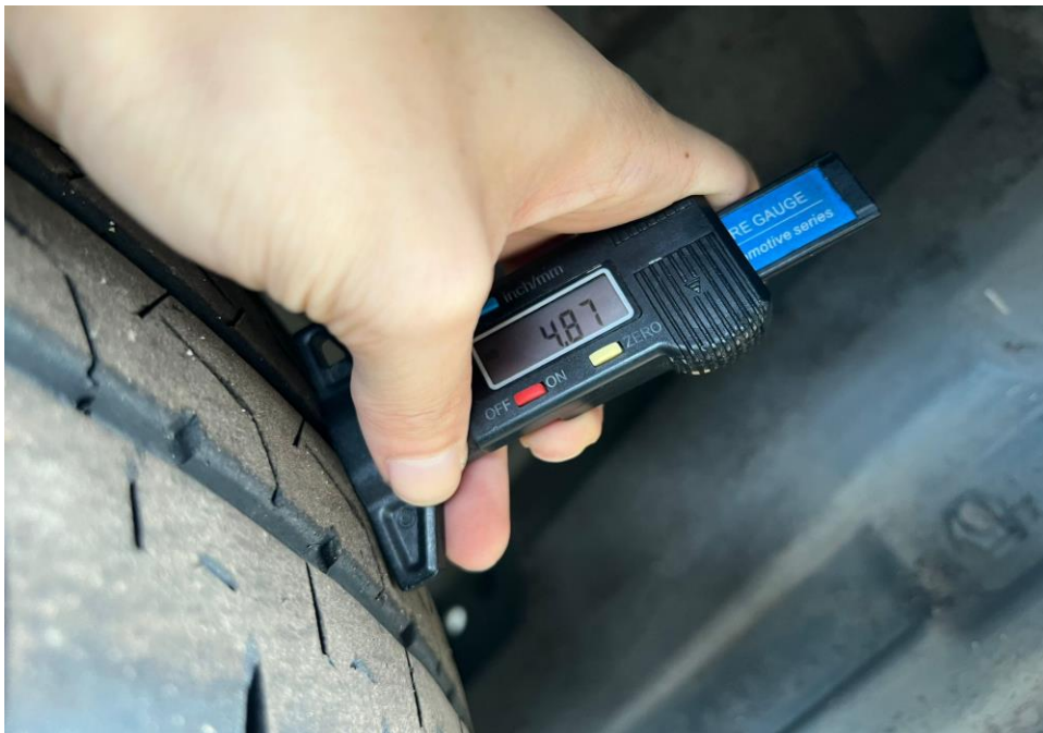
Photo 7 shows the tread depth of the front left tyre on the insured vehicle at the time of my inspection. The remaining tread depth is 4.8mm which is within the LTA requirements.
