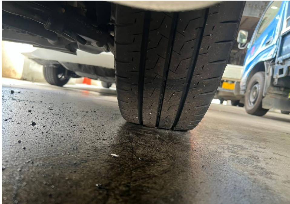
Photo 6 shows front right tyre of the insured vehicle at the time of my inspection. The front right tyre of the insured vehicle was observed to be in serviceable condition with remaining tread depth of 4.4mm which is within LTA requirements.
