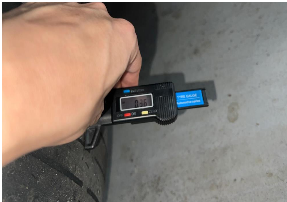
Photo 14 shows the tread depth of the rear left outer tyre (inner tread) on the insured vehicle at the time of my inspection. The remaining tread depth is 0.3mm which is not within the LTA requirements.
