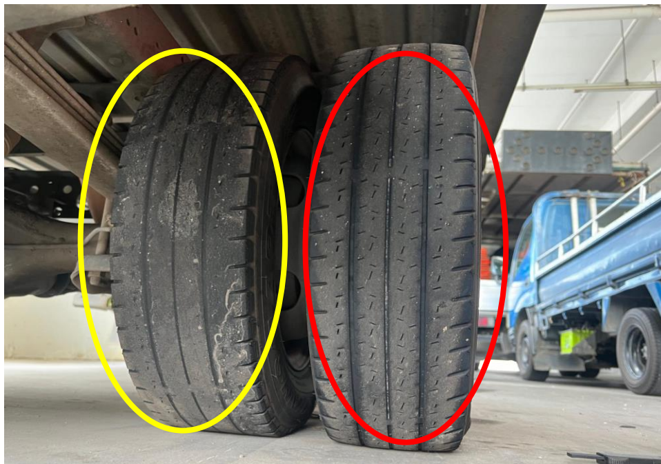
Photo 11 shows rear right tyre tyres of the insured vehicle at the time of my inspection. The rear right tyres of the insured vehicle was observed to be in serviceable condition with remaining tread depth of 2.0mm on the rear right outer tyre (red circle) and 1.4mm on the rear right inner tyre (yellow circle) which is within LTA requirements.
