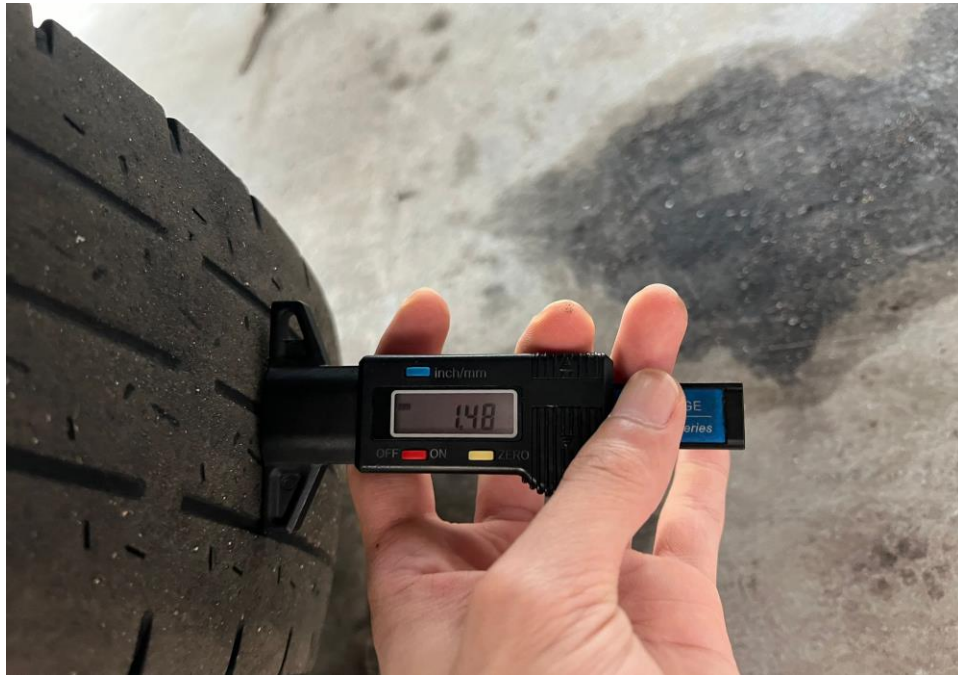
Photo 10 shows the tread depth of the rear right inner tyre on the insured vehicle at the time of my inspection. The remaining tread depth is 1.4mm which is within the LTA requirements.
