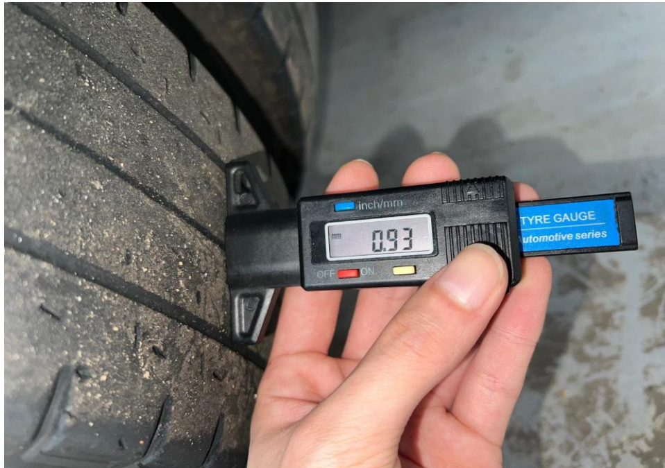
Photo 13 shows the tread depth of the rear left outer tyre (centre tread) on the insured vehicle at the time of my inspection. The remaining tread depth is 0.9mm which is not within the LTA requirements.
