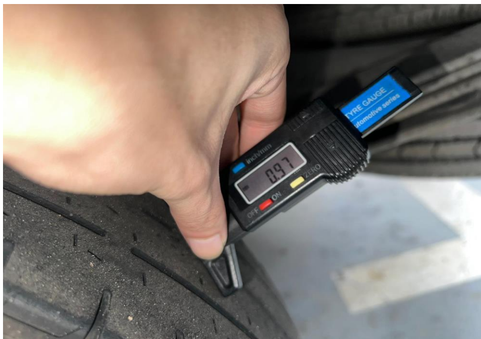
Photo 16 shows the tread depth of the rear left inner tyre (centre tread) on the insured vehicle at the time of my inspection. The remaining tread depth is 0.4mm which is not within the LTA requirements.
