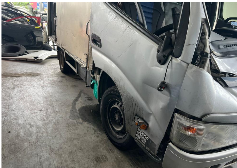
Photo 2 shows the close up view of the right of the insured vehicle at the time of my inspection. Its front right door was observed to be damaged as a result of the accident.
