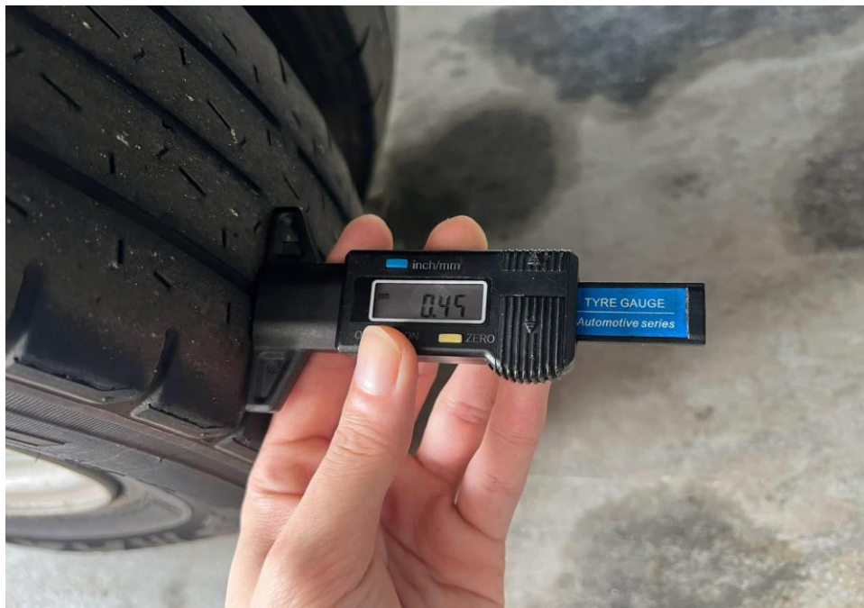
Photo 12 shows the tread depth of the rear left outer tyre (outer tread) on the insured vehicle at the time of my inspection. The remaining tread depth is 0.4mm which is not within the LTA requirements.
