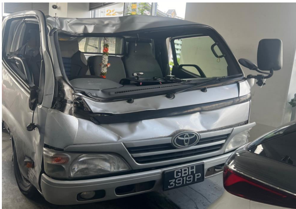
Photo 1 shows a general view of the Insured Vehicle front portion at the time of my inspection. The Insured Vehicle was observed to have sustained damage at its front portion. Its front windscreen, front body panel, front left headlamp and front bumper was amongst the body parts damaged as a result of the accident.
