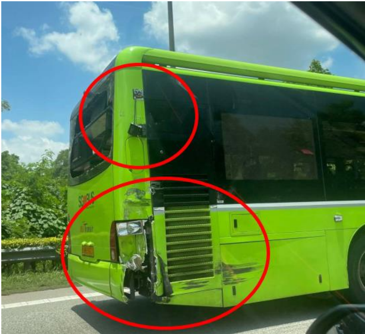
Figure B-12: Close-up View of Damages to SMB2161J
