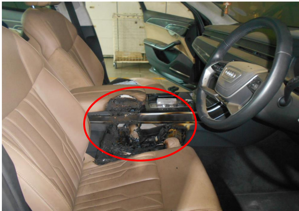
Photo 6 shows the general view of the interior compartment of the Insured Vehicle at the time of our inspection. Parts and components (circled) that had sustained fire/smoke damage
