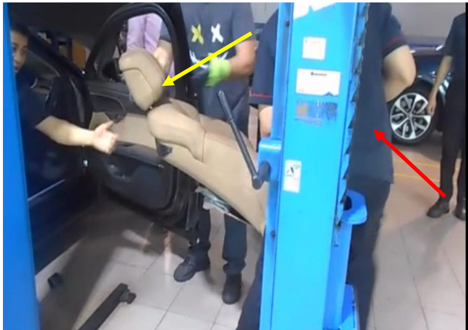
Photo 16 shows the technician at PA (red arrow) removing the driver seat (yellow arrow).
