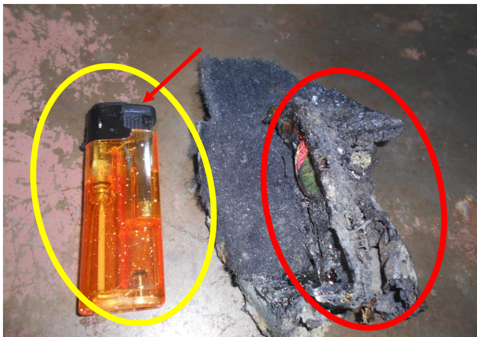
Photo 25 shows the close up view of the burnt cigarette lighter (red circle) that was removed from the Insured Vehicle's placed alongside a cigarette lighter that we believe to be similar type. (yellow circle). The head of the cigarette lighter (red arrow) had flicked into an "open" position when the driver's seat had electronically moved backwards automatically (due to easy access feature). This had caused the lighter to ignite flames, ultimately leading to the fire to the interior compartment of the Insured Vehicle.
