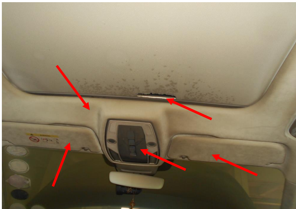
Photo 10 shows the general view of the interior roof headliner trim of the Insured Vehicle at the time of our inspection. The surfaces had suffered heat and smoke damages (red arrows) as a result of the fire.
