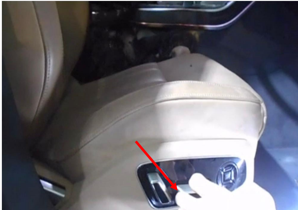
Photo 13 shows the drive electric power seat controls being pushed towards the seat incline position (red arrow) during the operational/functionality test.
