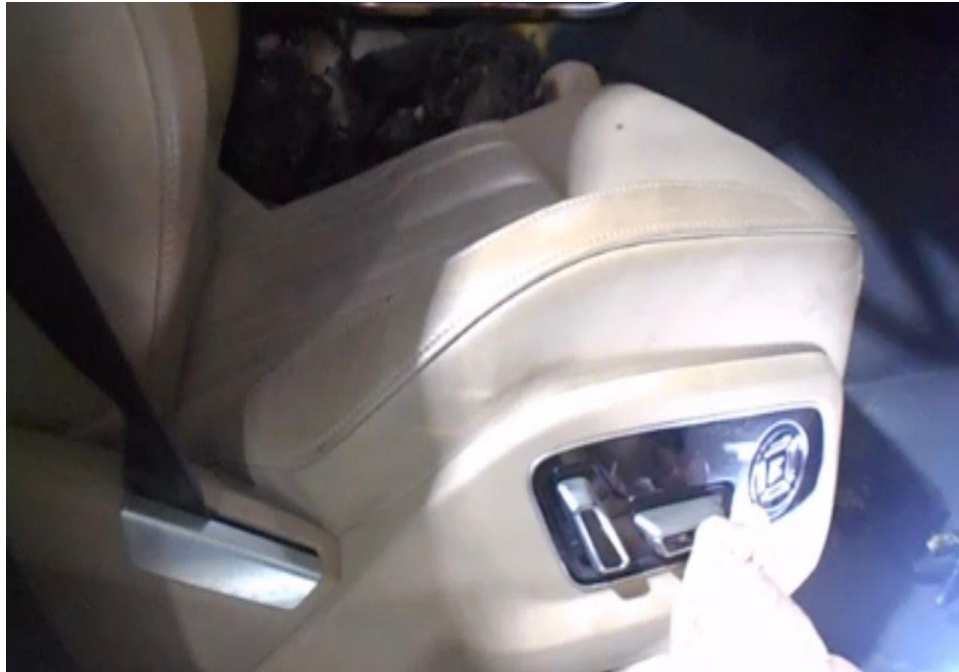
Photo 11 shows the driver electric power seat controls being pushed towards the seat decline position (red arrow) during the operational/functionality test.
