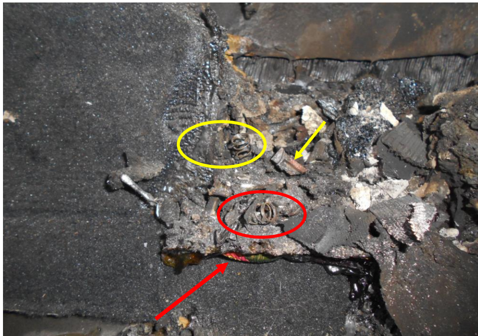
Photo 20 shows a close up view of the driver seating compartment of the Insured Vehicle upon dismantling the driver seat. Its front right foot well where reminiscent of a burnt cigarette lighter (red arrow) along with components of the cigarette lighter such as the fork spring (red circle), flint spring (yellow circle) and flint ignitor (yellow arrow) was found within the vicinity of the driver footwell/seat railing area.
