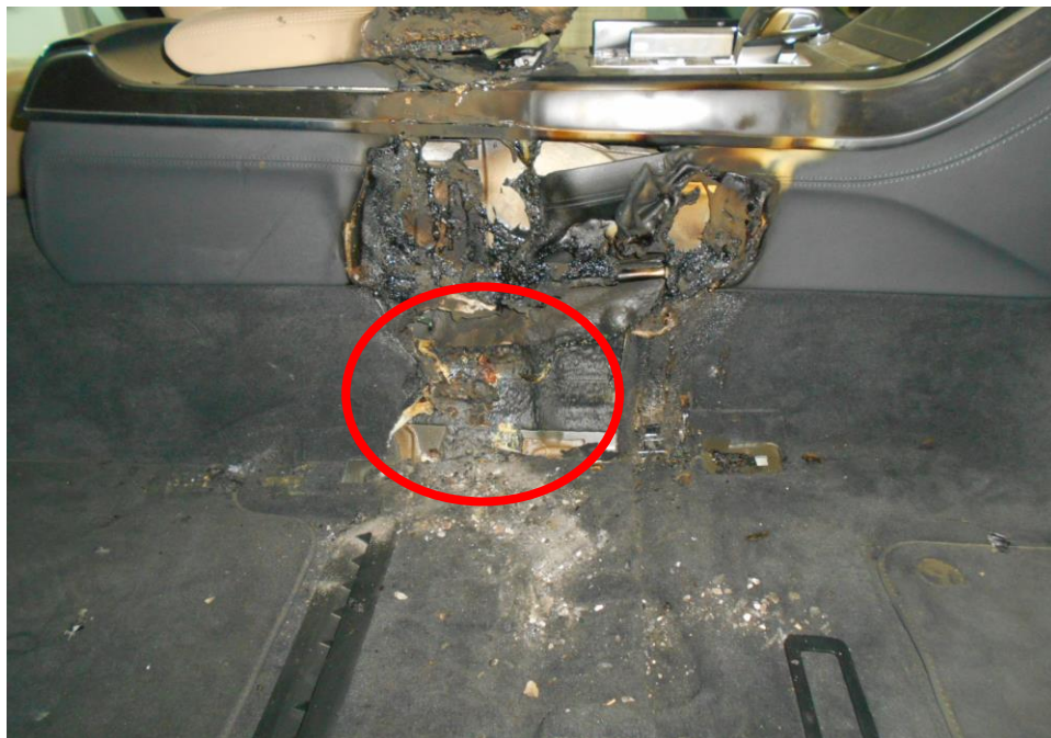
Photo 19 shows a general view of the driver seating compartment of the Insured Vehicle upon dismantling the driver seat. Its front right foot well (circled) where remains of a burnt cigarette lighter along with components of the cigarette lighter such as the fork spring, flint spring and flint ignitor was found within the vicinity of the driver footwell/seat railing area.
