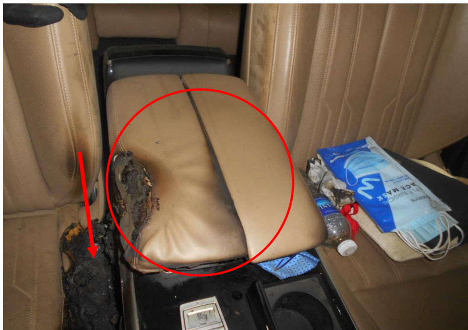
Photo 7 shows the close up view of the from the driver seating compartment of the Insured Vehicle at the time of our inspection. Its centre console armrest (red circle) and front right driver seat (red arrow) was found to have been burnt and melt as a result of the fire.
