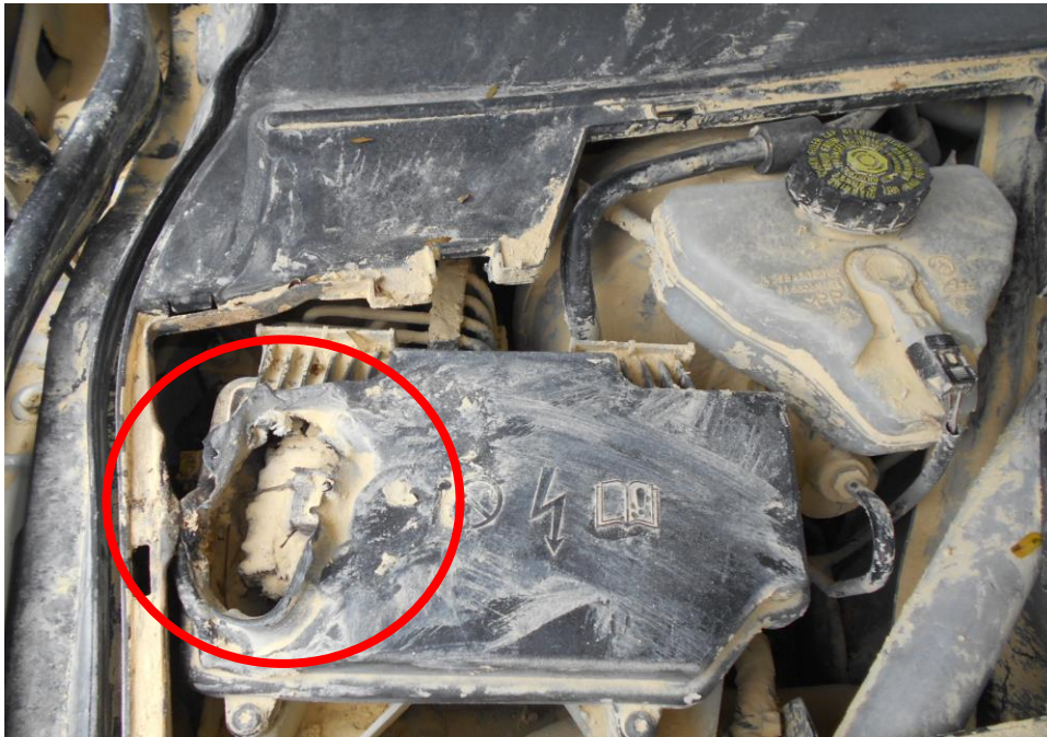
Photo 8 shows the general view of the Engine Fuse and Relay box upon removing the top plastic cover located at the rear right of the engine bay. The Engine Fuse and Relay Box had sustained visible fire damages resulting in a hole found on the Engine Fuse and Relay Box (red circle).
