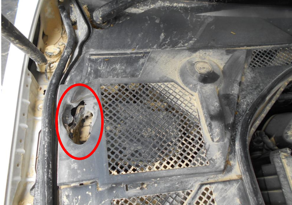
Photo 7 shows the general view of the Engine Fuse and Relay box top plastic cover located at the rear right of the engine bay which had sustained visible fire damages resulting in a hole found on the Engine Fuse and Relay Box top plastic cover (red circle).
