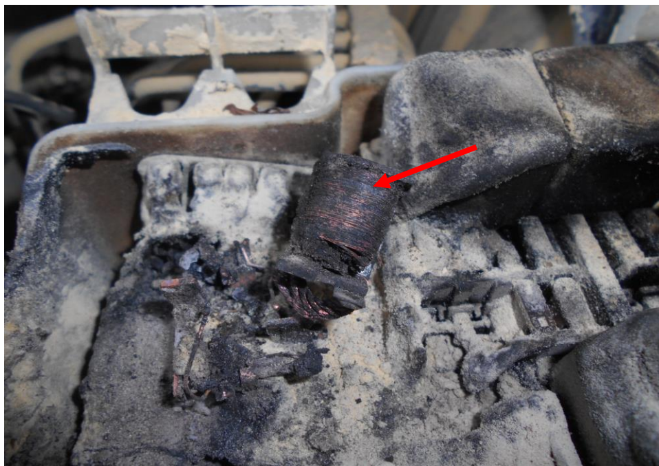
Photo 11 shows the close up view of the Engine Fuse and Relay along with the original fitted wirings found in the relay. The presence of greenish residue (red arrow) indicates internal heating of copper wires, a sign of an electrical short circuit occurring. The greenish residue is normally left behind from oxidation as a result of chemical reaction involving the copper wires.
