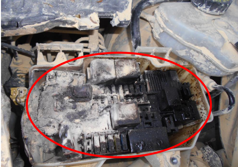
Photo 9 shows the general view of the Engine Fuse and Relay box upon removing the top plastic cover and exposing the Engine Fuse and Relays located at the rear right of the engine bay. The Engine Fuse and Relays had sustained visible fire damages at the time of my inspection (red circle).
