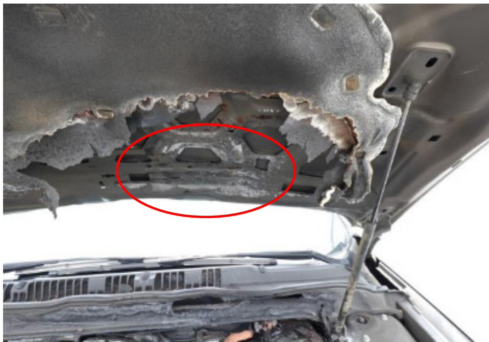
Photo 6 shows the burn pattern and whitish burn marks that were found on the underside of the front bonnet of the Insured Vehicle, at the bottom portion (circled). Such whitish burn marks are a result of exposure to prolonged heat intensity, which may indicate where the fire had started. Rust would also begin to develop on these areas soon after the fire.
