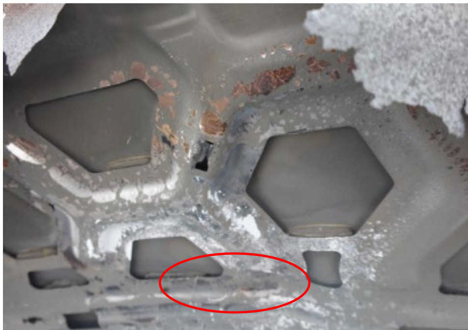
Photo 7 shows the rust that had developed on the underside of the front bonnet, around the bottom portion (circled). The development of rust is an indication that this area was subjected to prolonged exposure to high heat intensity, which had caused the steel/metal material of the front bonnet to be exposed to natural environmental condition. Hence the fire to the Insured Vehicle can be determined to have originated towards the rear portion of the engine compartment.
