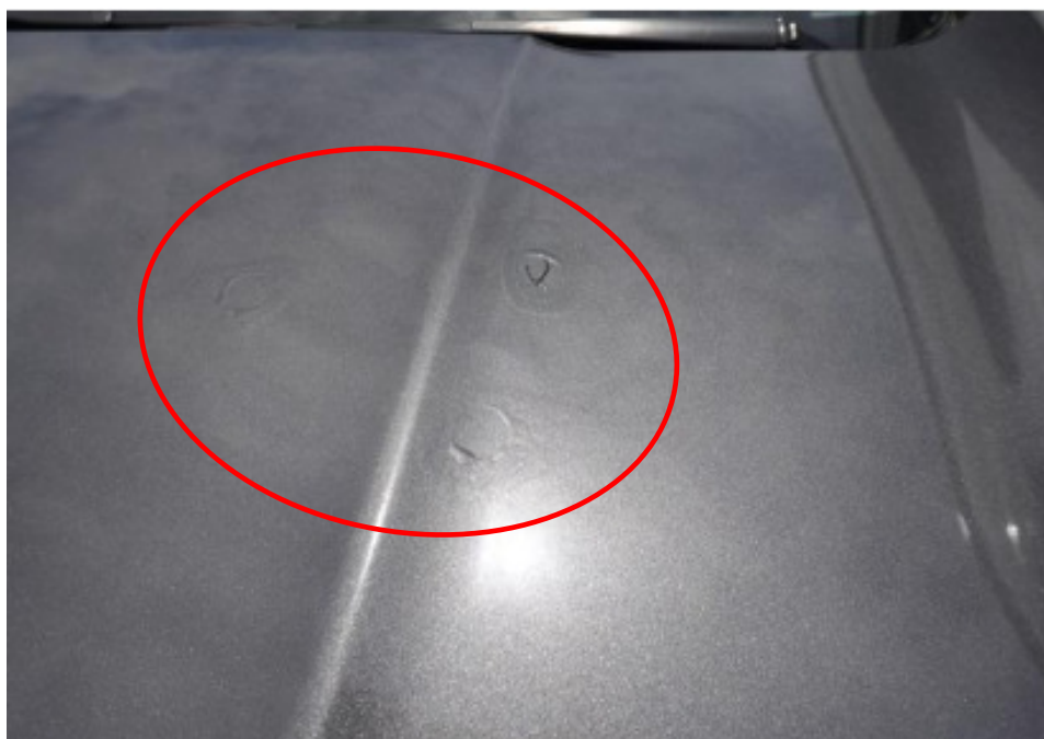
Photo 8 shows paint bubbles on the rear portion of the front bonnet (circled).
