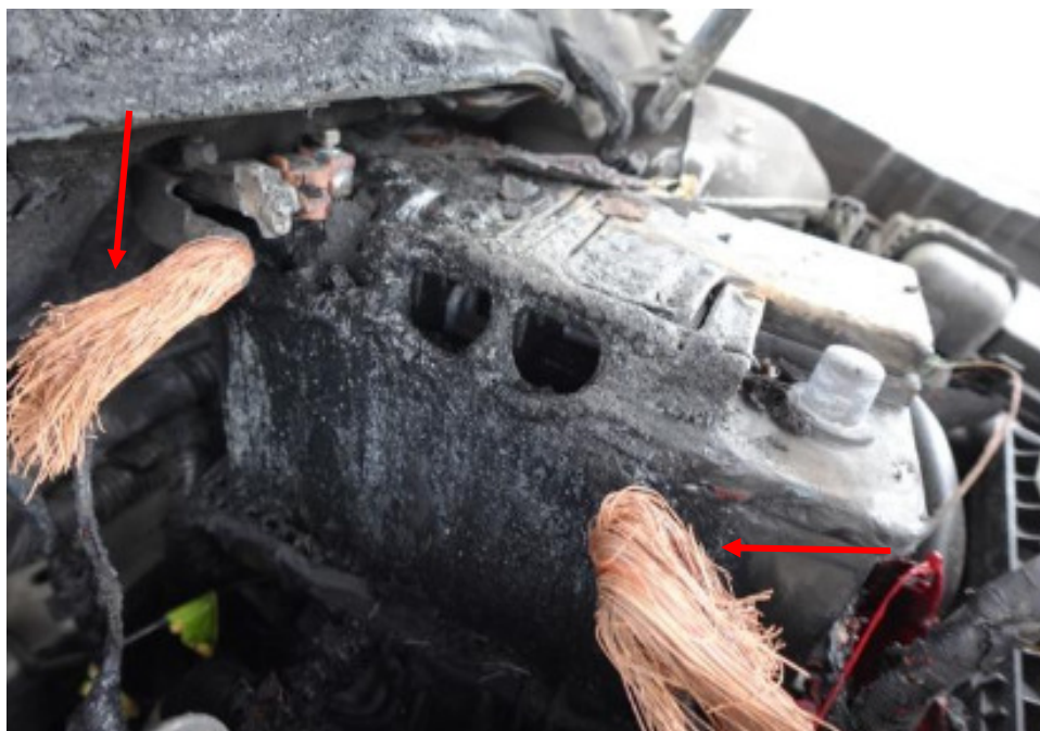
Photo 11 shows a close up view of the wirings leading from the battery (red arrows) which were found to have been burnt internally to its bare copper state, suggesting occurrence of an electrical short circuit.
