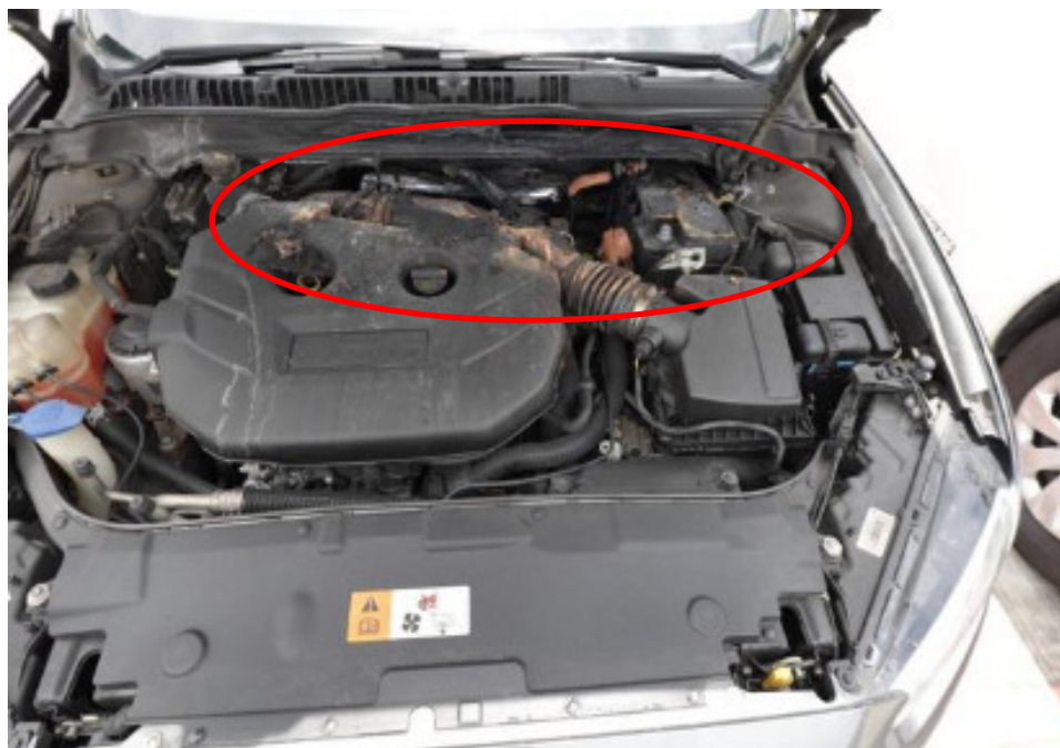
Photo 4 shows the general view of the engine compartment of the Insured Vehicle at the time of our inspection. The fire damage was confined to rear portion as observed by the burnt nature of the engine components towards the rear portion of the engine (circled).
