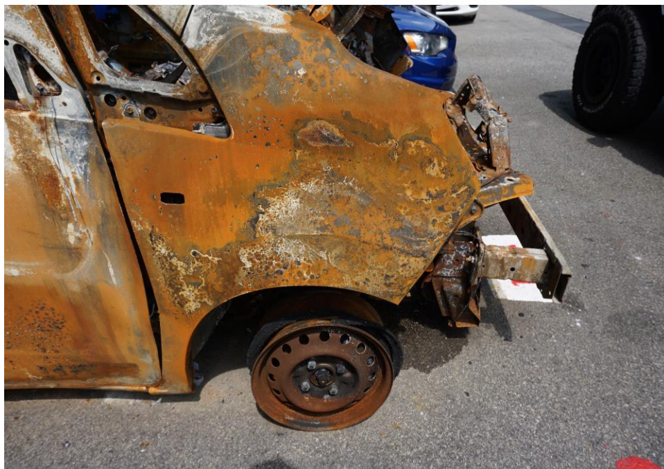
Photo 8 shows the front right fender of the Insured Vehicle at the time of our inspection. The High heat intensity burn marks (whitish burn marks) and rust that had development found on the exterior surface of the front right fender indicates that the fire had originated from the front right portion of the Insured Vehicle.
