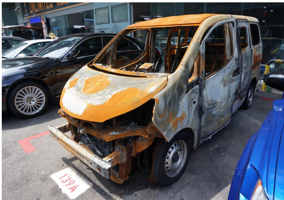
Photo 3 shows the general view of the left body of the Insured Vehicle at the time of our inspection. The Insured Vehicle was observed to have sustained extensive fire damage all around. Rust had accumulated all around the Insured Vehicle as a result of exposure to environmental condition for a period of time.
