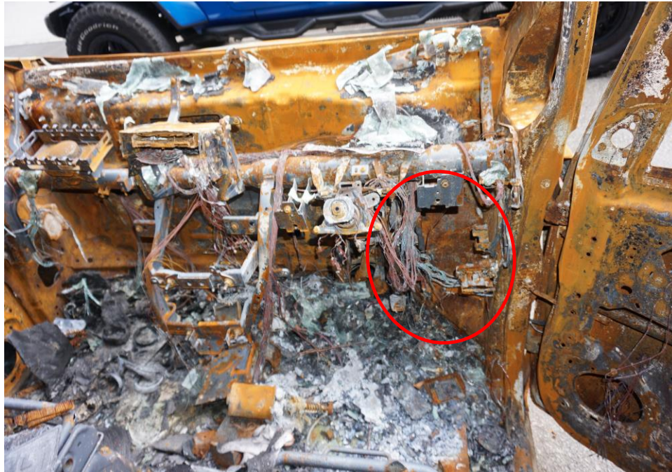
Photo 9 shows the general view of the driver interior compartment of the Insured Vehicle at the time of our inspection. We had observed that the driver's right portion (circled) had sustained a stronger high heat intensity burn marks.
