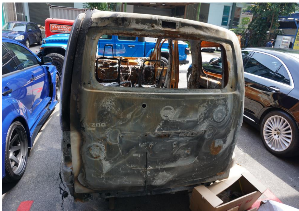
Photo 4 shows the general view of the rear portion of the Insured Vehicle. The Insured Vehicle was observed to have sustained extensive fire damage all around. Rust had accumulated all around the Insured Vehicle as a result of exposure to environmental condition for a period of time.
