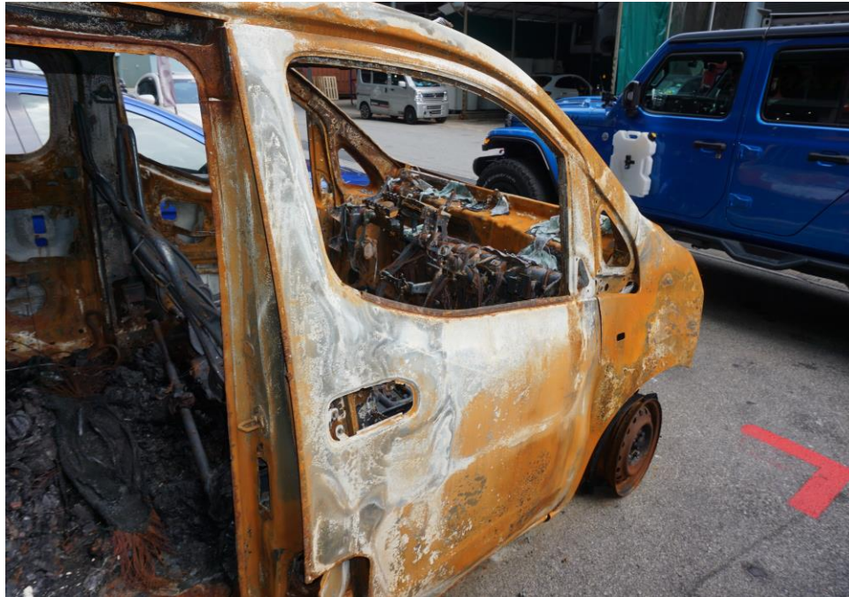
Photo 7 shows the exterior of the front right portion of the Insured Vehicle at the time of our inspection. The high heat intensity burn marks (whitish burn marks) and rust that had development found on the exterior surface of the bonnet indicates that the fire had originated from the front right portion of the Insured Vehicle.
