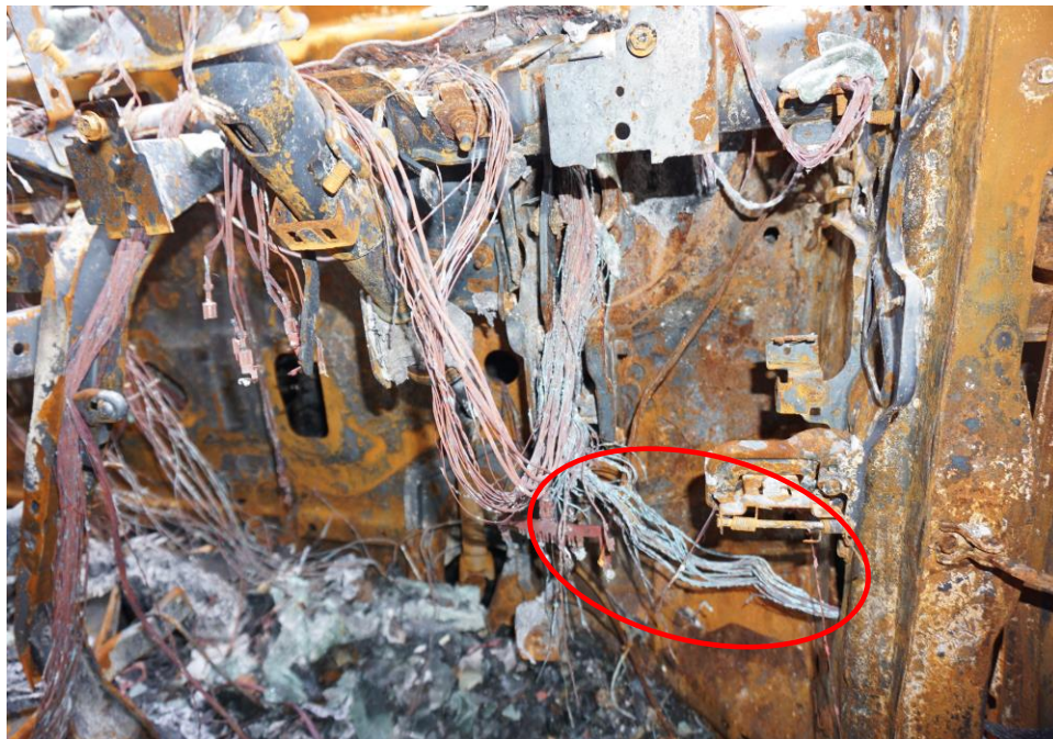
Photo 10 shows the close up view of the driver interior compartment of the Insured Vehicle at the time of our inspection. We had observed that the driver's right portion we had also found traces of greenish residue on the wirings harnesses (circled) leading from the battery to the electrical components in the cabin of the Insured Vehicle.
