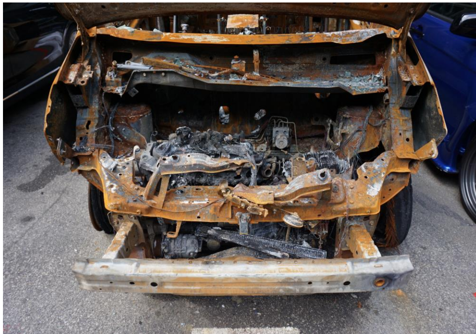
Photo 6 shows the engine compartment of the Insured Vehicle at the time of our inspection. The entire engine compartment of the Insured Vehicle was observed to be severely burnt. Most of the parts inside the engine compartment were found to be burnt and/or melted as a result of the fire.
