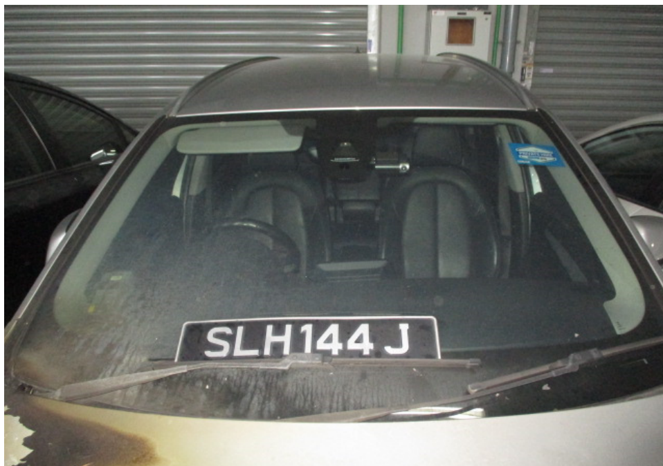
Photo 4 shows the general view of the front windscreen of the Insured Vehicle at the time of our inspection. The front windscreen had sustained serious fire damage.
