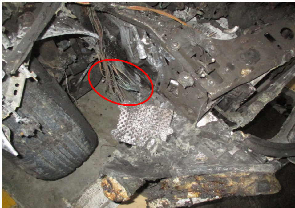
Photo 7 shows the wirings around the right frontal portion of the engine compartment, which is in the immediate vicinity where the fire to the Insured Vehicle had likely started. We noticed greenish residue on several stretches of burnt wirings (circled). The presence of greenish residue indicates internal heating of copper wires, a sign of an electrical short circuit occurring.
