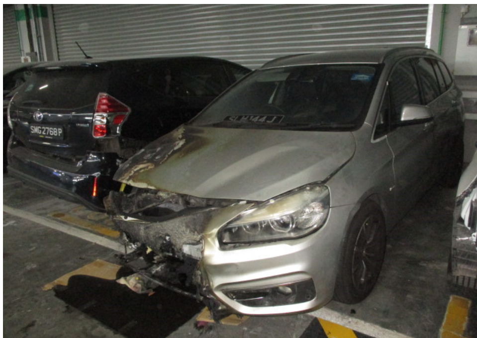
Photo 2 shows the general view of the left front body of the Insured Vehicle at the time of our inspection. The fire damage to the Insured Vehicle was confined to its frontal portion. The entire engine compartment of the Insured Vehicle was observed to be severely burnt while the interior compartment was observed to be relatively unaffected by the fire.
