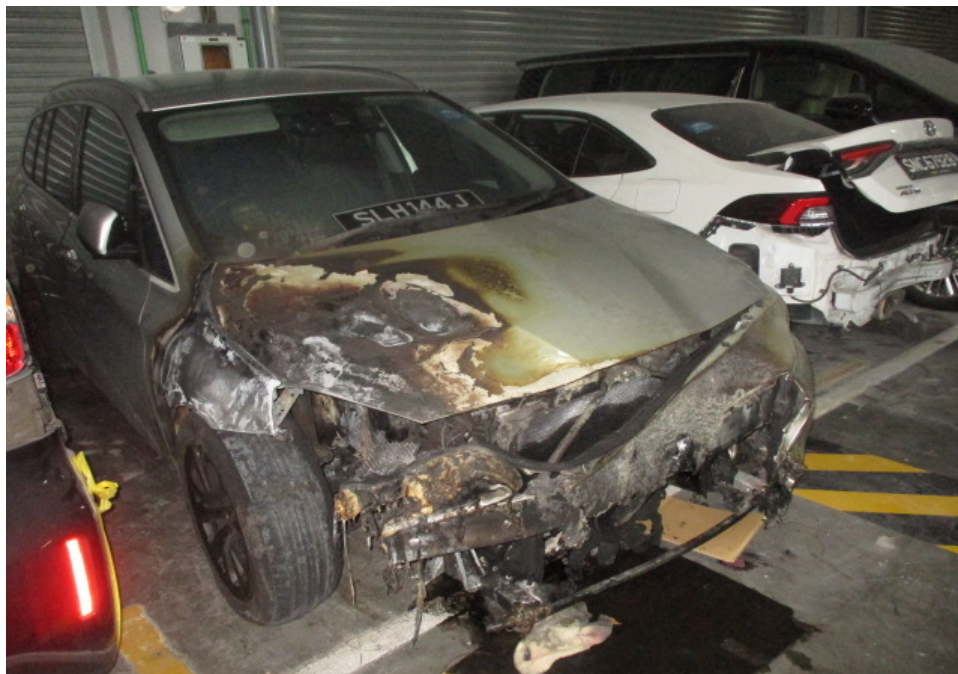
Photo 3 shows the closer view of the right front body of the Insured Vehicle at the time of our inspection. The fire damage to the Insured Vehicle was confined to its frontal portion. Its front bumper, front bonnet, front support panel, front grille, headlamps, front windscreen, front wheel rims, front fenders and front tyres, amongst others were amongst the body parts that were found to have been affected by the fire.
