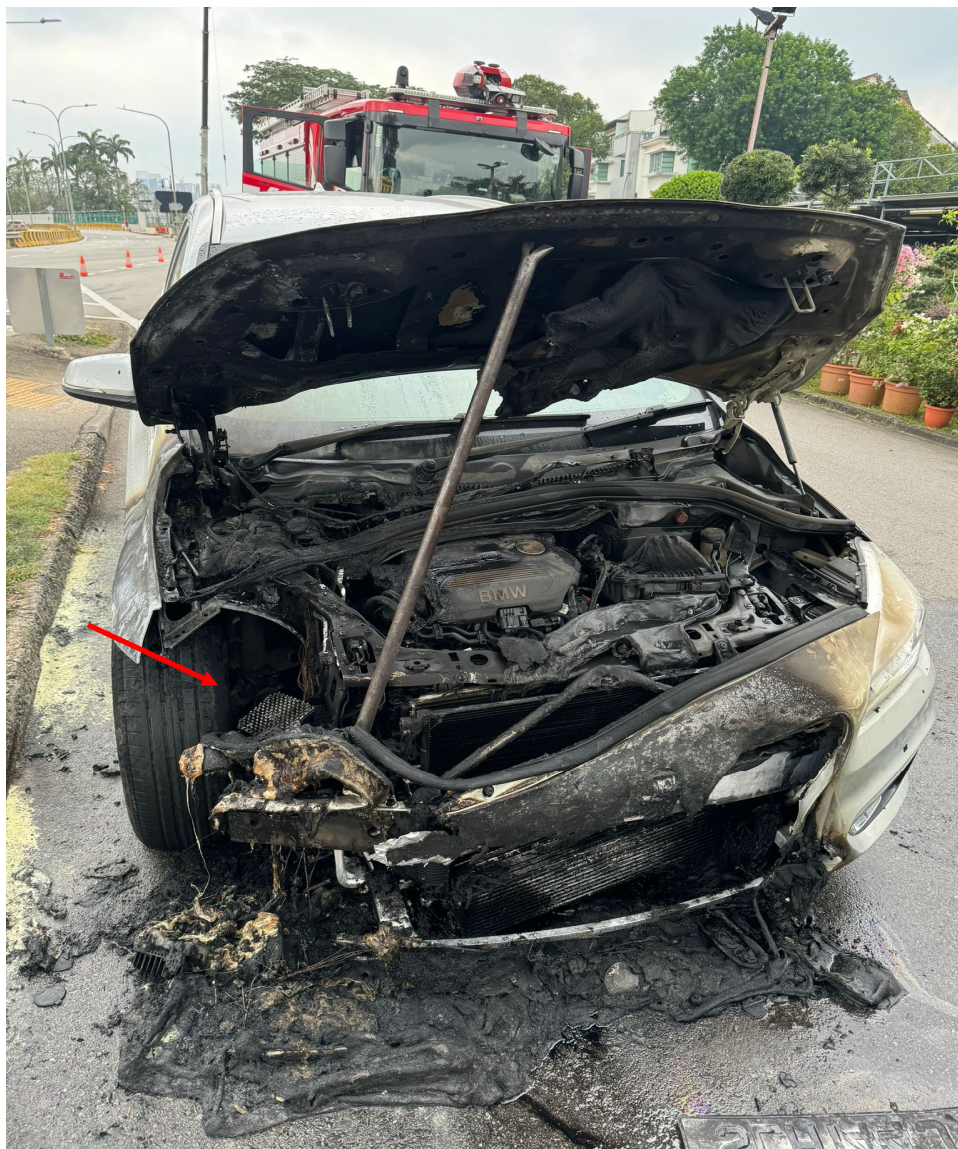
Photo 13 shows the Insured Vehicle post- incident. In general, the information that could be gathered from this photograph had corresponded to the events that were related to us by Mr Kong which is the fire had started from the engine compartment of the Insured Vehicle (arrowed).
