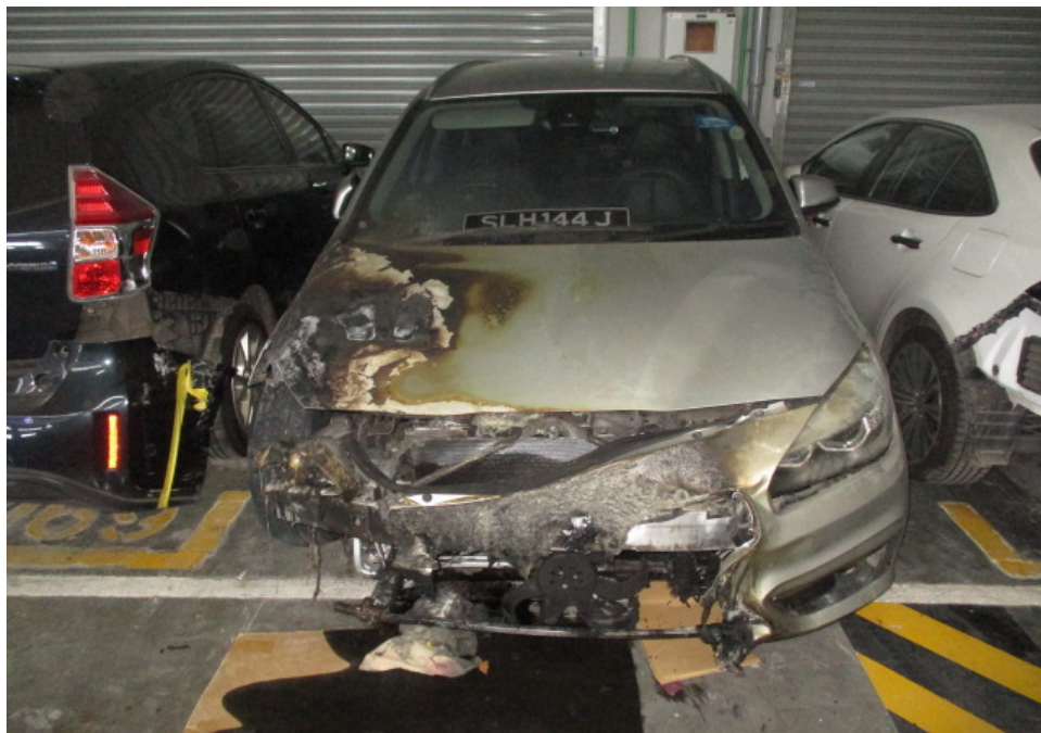
Photo 1 shows the general view of the frontal portion of the Insured Vehicle at the time of our inspection. The fire damage to the Insured Vehicle was confined to its frontal portion.
