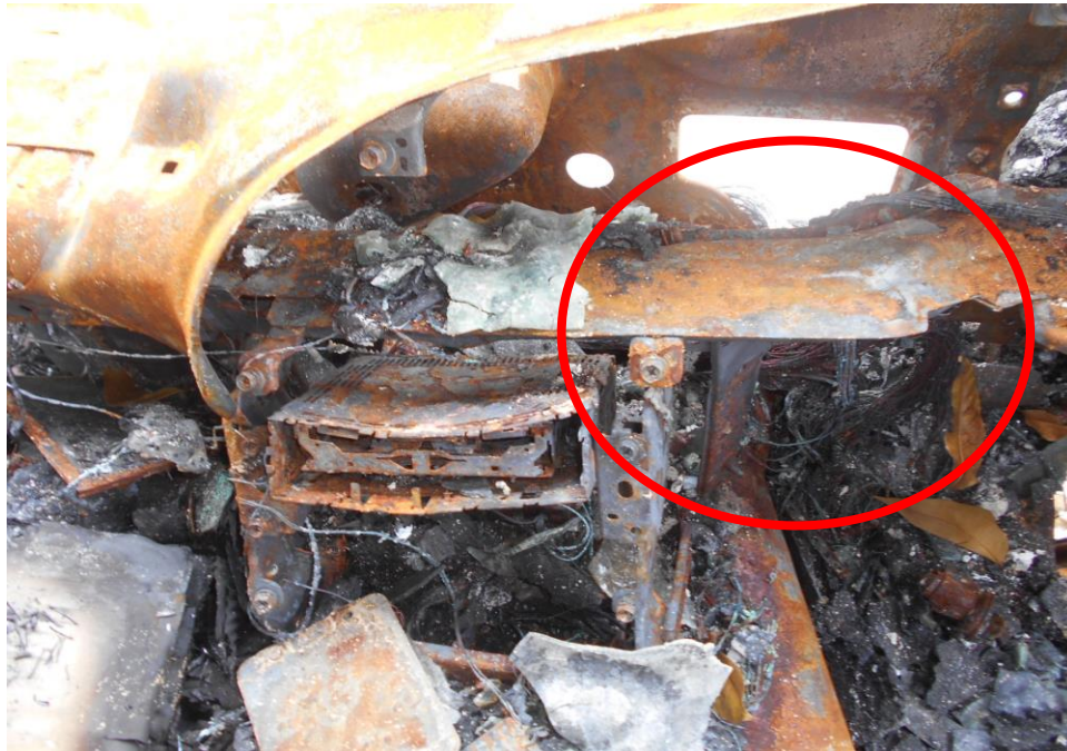
Photo 7 shows the burnt wirings around the front right driver portion of the interior dashboard which is near to the vicinity where the fire to the Insured Vehicle had likely started (circled).
