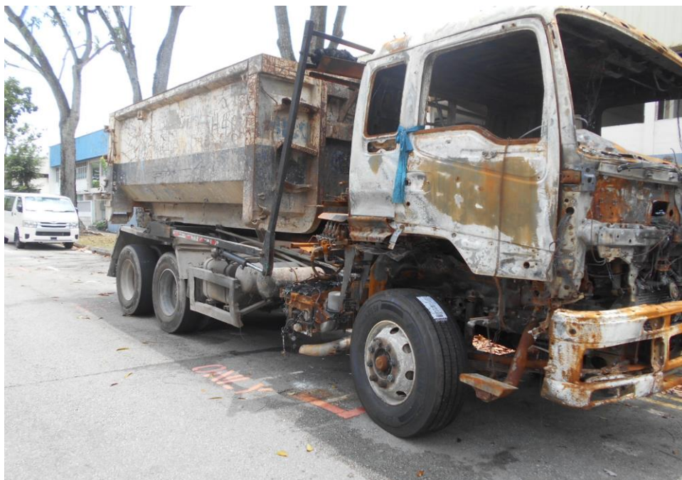
Photo 2 shows the general view of the right body of the Insured Vehicle at the time of our inspection. The exterior of the Insured Vehicle had sustained visible fire damages. This included its side panels and front right door.
