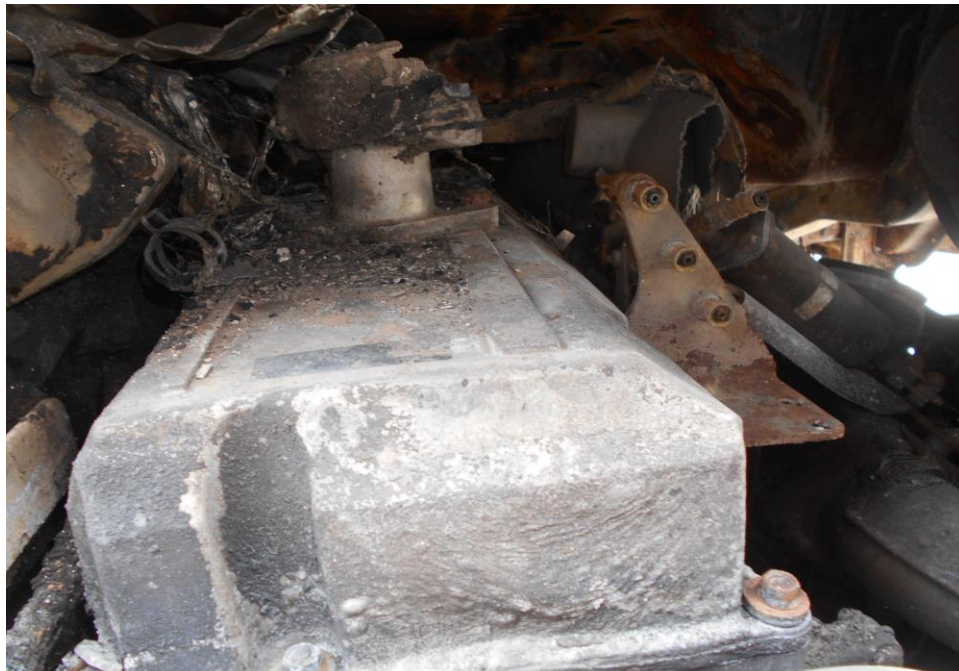
Photo 6 shows the general view of the engine portion of the Insured Vehicle at the time of our inspection. The fire damage to the Insured Vehicle was confined to its interior and exterior portion. Its engine compartment is observed to be unaffected by the fire.
