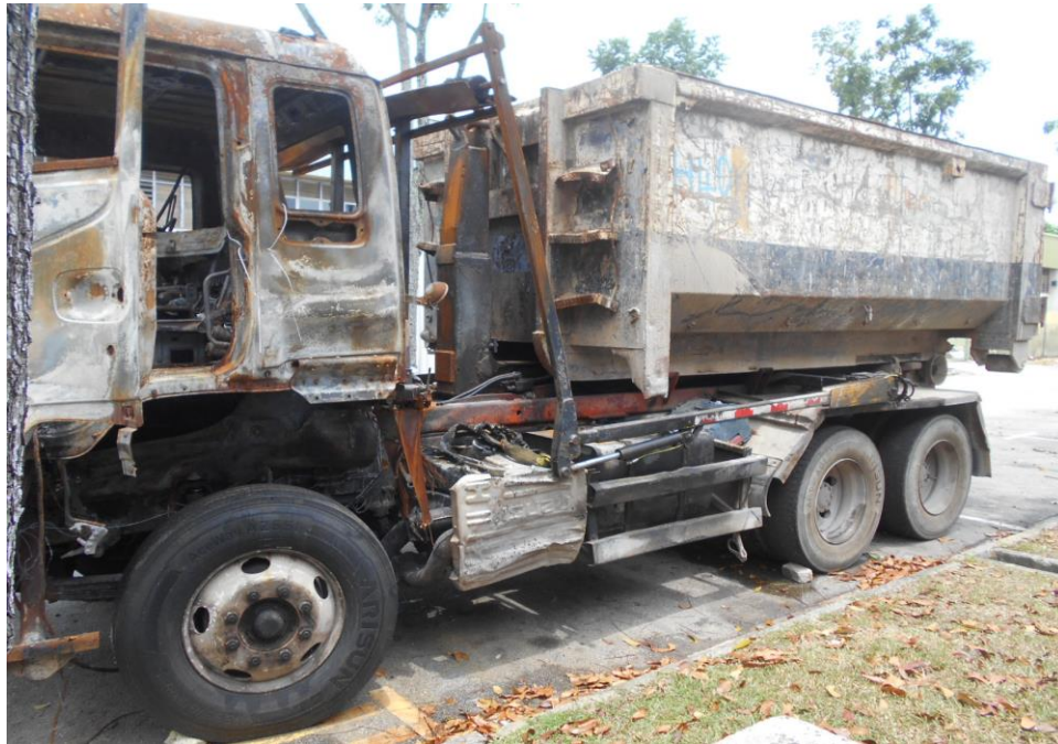
Photo 3 shows the general view of the left body of the Insured Vehicle at the time of our inspection. The exterior of the Insured Vehicle had sustained visible fire damages. This included its side panels and front left door.
