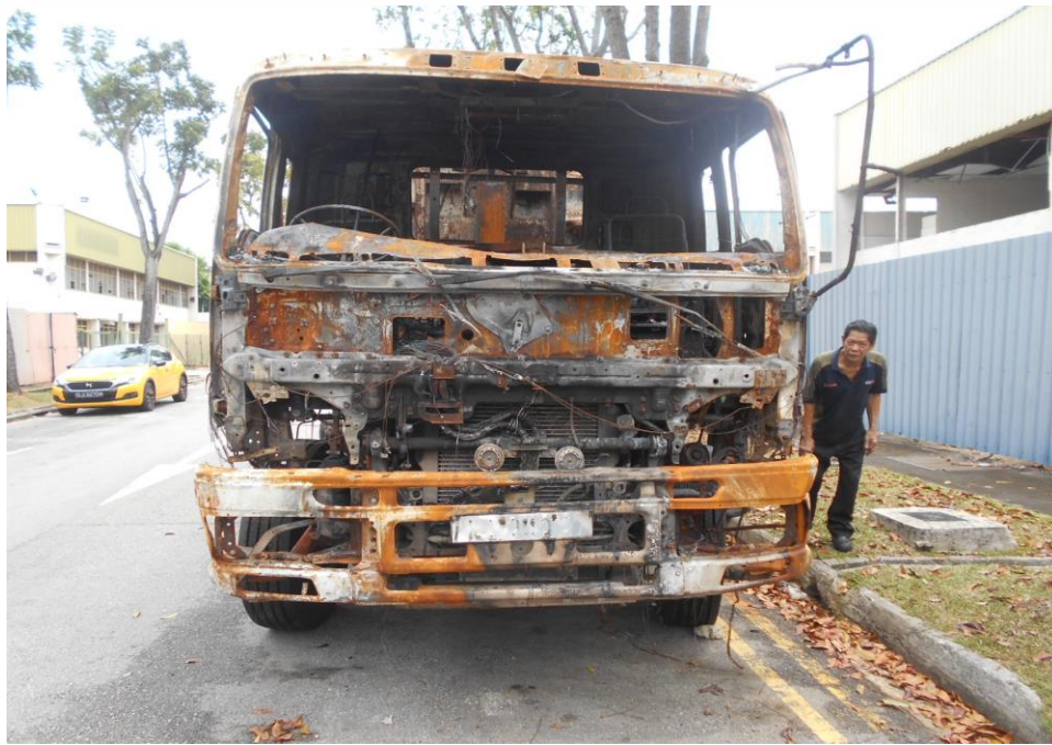
Photo 1 shows the general view of the frontal portion of the Insured Vehicle at the time of our inspection. The exterior of the Insured Vehicle had sustained visible fire damage. This included its front windscreen, front body panels and headlights.
