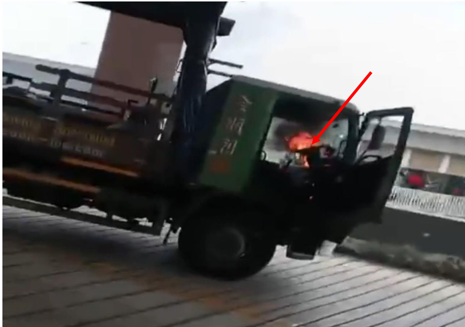
Photo 11 shows flames emitting from the centre dashboard of the Insured Vehicle interior compartment. (red arrow).
