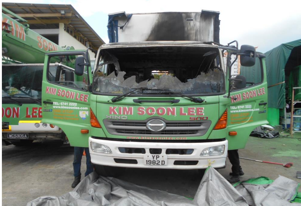
Photo 1 shows the general view of the frontal portion of the Insured Vehicle at the time of our inspection. The exterior of the Insured Vehicle had sustained visible fire damages. This included its front windscreen.
