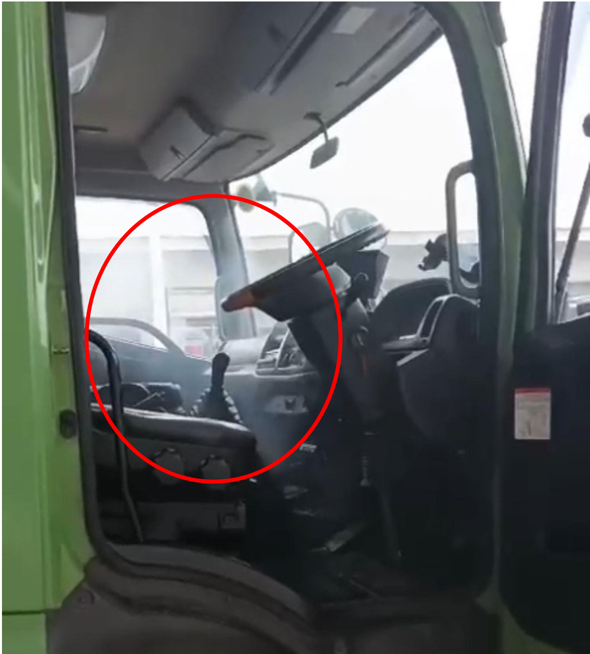
Photo 10 shows white smoke emitting from the centre dashboard of the Insured Vehicle interior compartment. (red circle).
