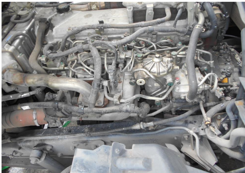
Photo 6 shows the general view of the engine portion of the Insured Vehicle at the time of our inspection. The fire damage to the Insured Vehicle was confined to its interior portion. Its engine compartment is observed to be unaffected by the fire.
