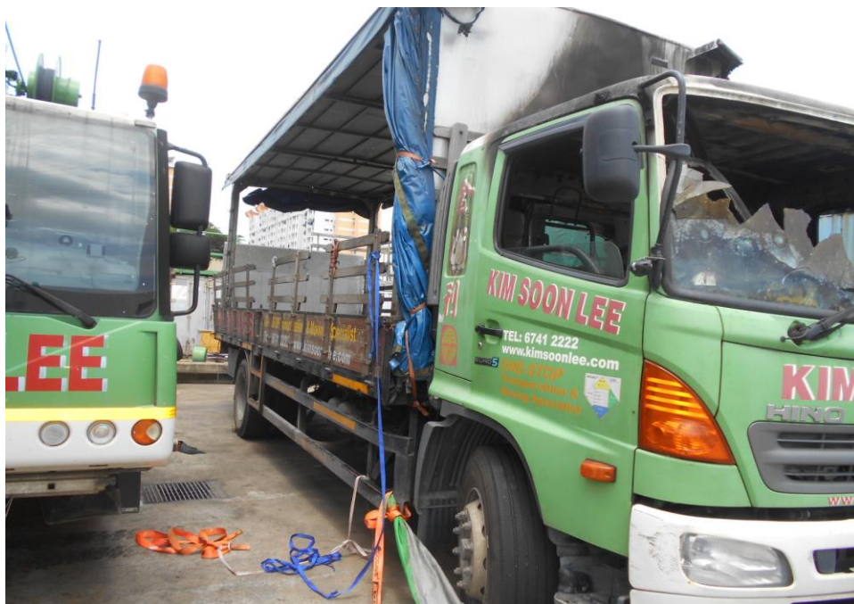
Photo 2 shows the general view of the right body of the Insured Vehicle at the time of our inspection. The exterior of the Insured Vehicle had sustained visible fire damages. This included its front right body panel.
