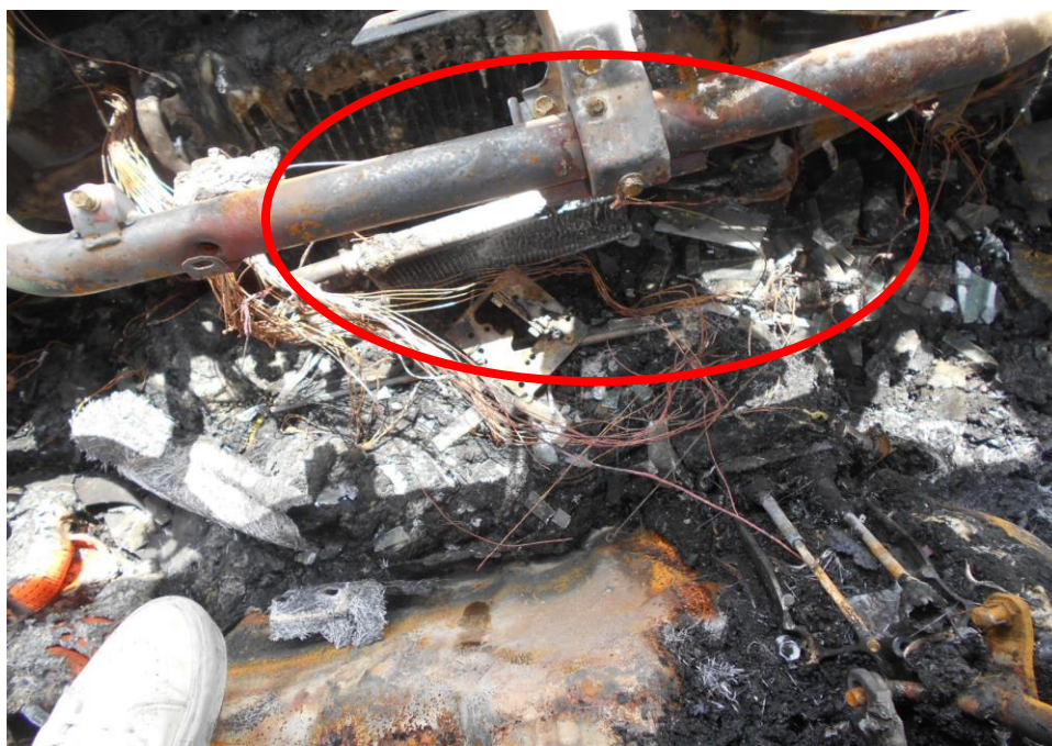
Photo 7 shows the burnt wirings around the front centre portion of the interior dashboard which is near to the vicinity where the fire to the Insured Vehicle had likely started (circled).
