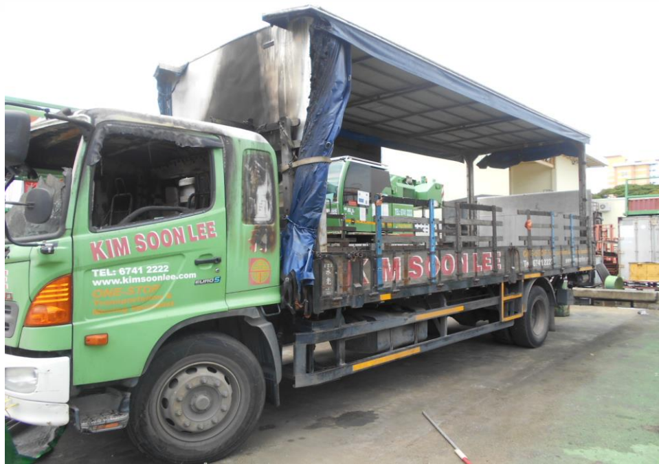
Photo 3 shows the general view of the left body of the Insured Vehicle at the time of our inspection. The exterior of the Insured Vehicle had sustained visible fire damages. This included its front left body panel.
