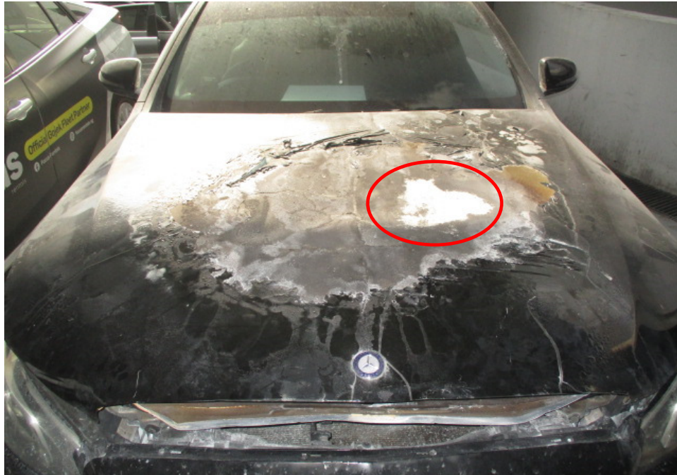
Photo 7 shows the burn pattern and whitish burn marks that were found on the centre portion of the front bonnet of the Insured Vehicle (circled). Such whitish burn marks are a result of exposure to prolonged heat intensity, which may indicate where the fire had started. Rust would also begin to develop on these areas soon after the fire.
