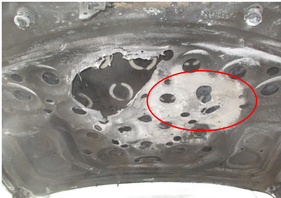
Photo 10 shows a closer view of the rust that had developed on the underside of the front bonnet, around the centre portion (circled).
