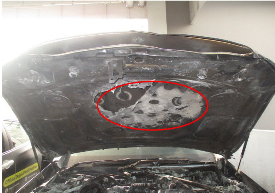
Photo 9 shows the rust that had developed on the underside of the front bonnet, around the centre portion (circled). The development of rust is an indication that this area was subjected to prolonged exposure to high heat intensity, which had caused the steel/metal material of the front bonnet to be exposed to natural environmental condition. Hence the fire to the Insured Vehicle can be determined to have originated towards the centre portion of the engine compartment.
