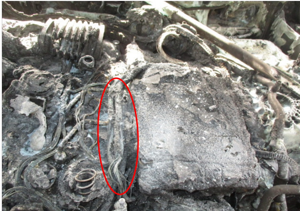
Photo 12 shows a closer view of the greenish residue on some of the burnt wirings of the Insured Vehicle (circled). The presence of greenish residue indicates internal heating of copper wires, a sign of an electrical short circuit occurring. The greenish residue is normally left behind from oxidation as a result of chemical reaction involving the copper wires.
