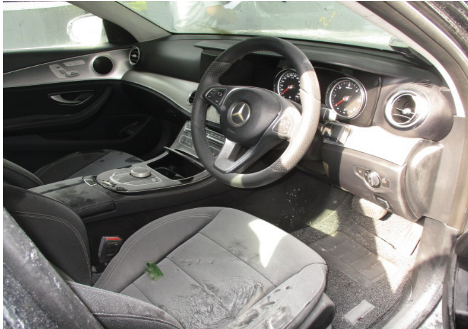
Photo 5 shows the interior compartment of the Insured Vehicle at the time of our inspection. The interior compartment of the Insured Vehicle was observed to be relatively unaffected by the fire.
