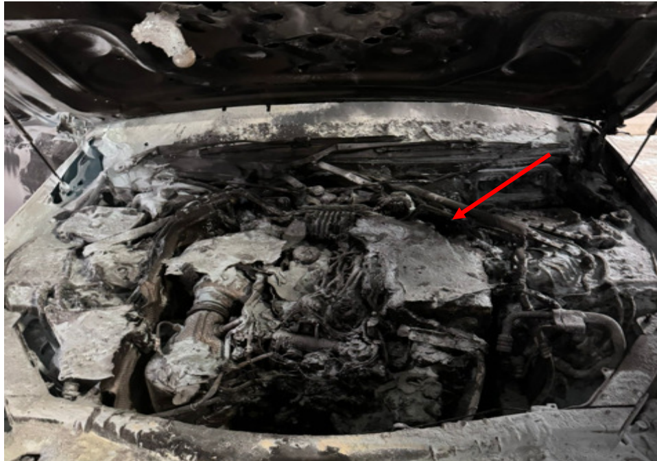
Photo 19 shows the engine compartment of the Insured Vehicle at the post-incident after the front bonnet was prised open by the SCDF. The severity of damage of the frontal portion had corresponded to the events that were related to us by Mr Ouyang, which is the fire had started from the engine compartment of the Insured Vehicle (arrowed).
