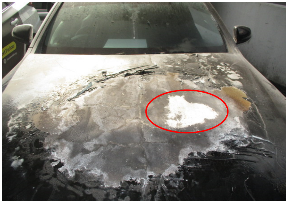
Photo 8 shows a closer view of the burn pattern and whitish burn marks that were found on the centre portion of the front bonnet of the Insured Vehicle (circled).
