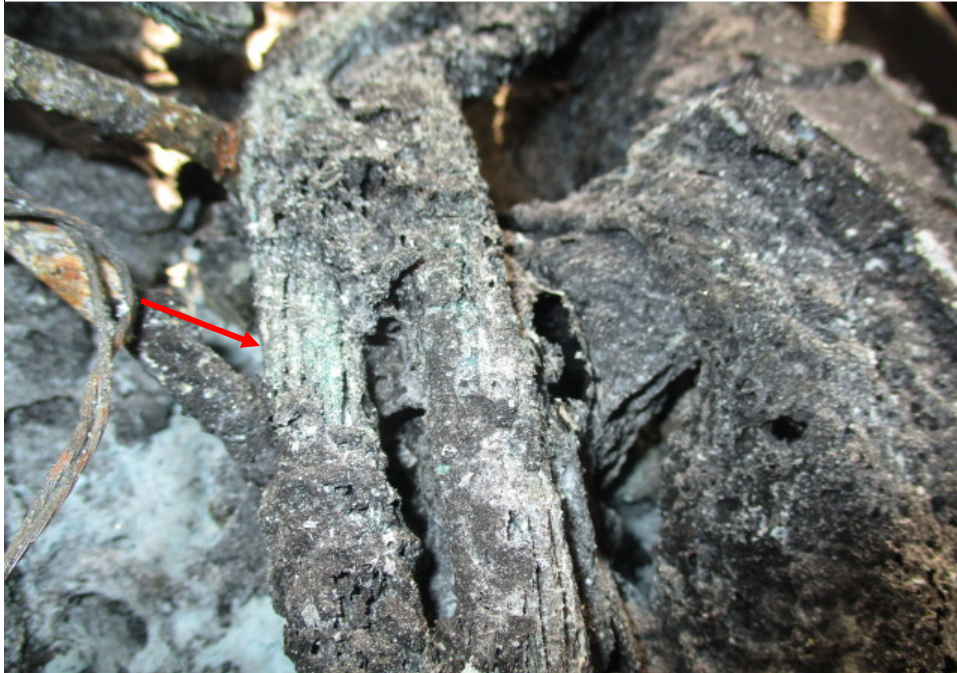
Photo 14 shows a close up view of the greenish residue on the wirings of the Insured Vehicle (arrowed). The presence of such greenish residue suggests occurrence of an electrical short circuit.
