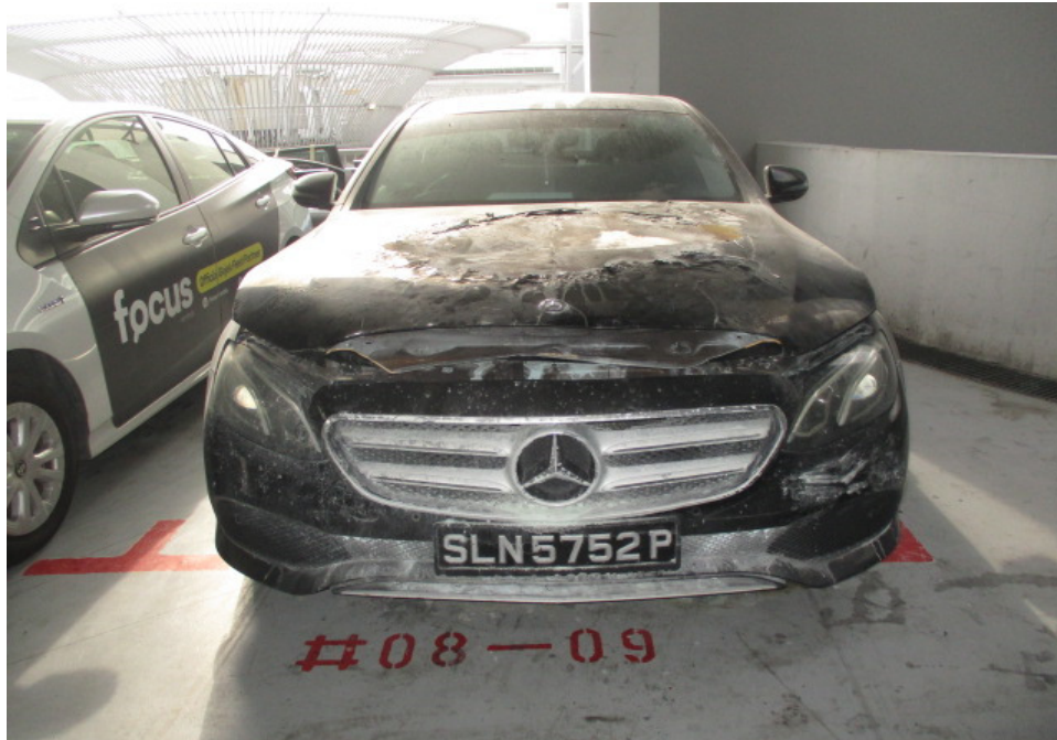
Photo 1 shows the general view of the frontal portion of the Insured Vehicle at the time of our inspection. The exterior body of the Insured Vehicle had sustained visible fire damage. This included its front windscreen, front bonnet, front windscreen wiper garnish, front windscreen wipers and front fenders.
