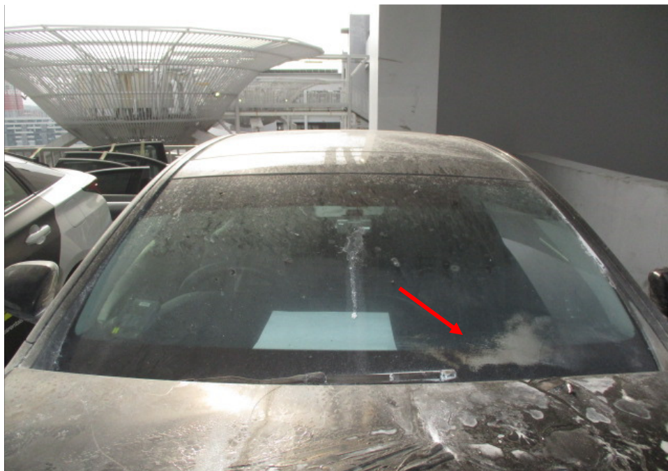
Photo 4 shows a closer view of the front windscreen of the Insured Vehicle at the time of our inspection. The front windscreen had sustained slight fire damage (arrowed).
