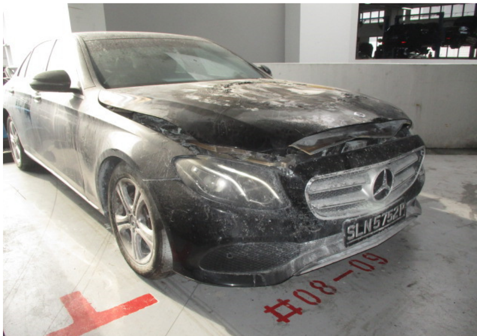
Photo 2 shows the general view of the right frontal portion of the Insured Vehicle at the time of our inspection. The exterior body of the Insured Vehicle had sustained visible fire damage. This included its front windscreen, front bonnet, front windscreen wiper garnish, front windscreen wipers and right front fender.
