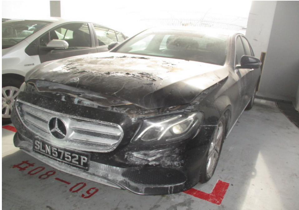
Photo 3 shows the general view of the left portion of the Insured Vehicle at the time of our inspection. The exterior body of the Insured Vehicle had sustained visible fire damage. This included its front windscreen, front bonnet, front windscreen wiper garnish, front windscreen wipers and left front fender.
