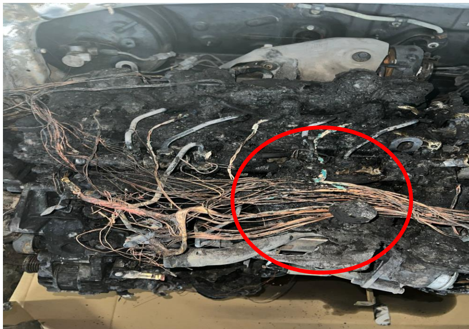
Photo 8 shows the burnt wirings around the front centre portion of the engine compartment which is near to the vicinity where the fire to the Insured Vehicle had likely started (circled).
