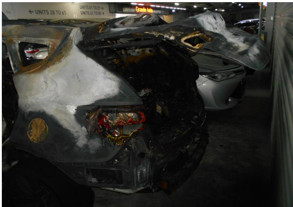
Photo 2 shows the general view of the rear portion of the Insured Vehicle at the time of our inspection. The Insured Vehicle was observed to have sustained extensive fire damage all around. Its engine compartment and interior compartment were completely burnt. Rust had accumulated all over the Insured Vehicle as a result of exposure to environmental condition for a period of time.
