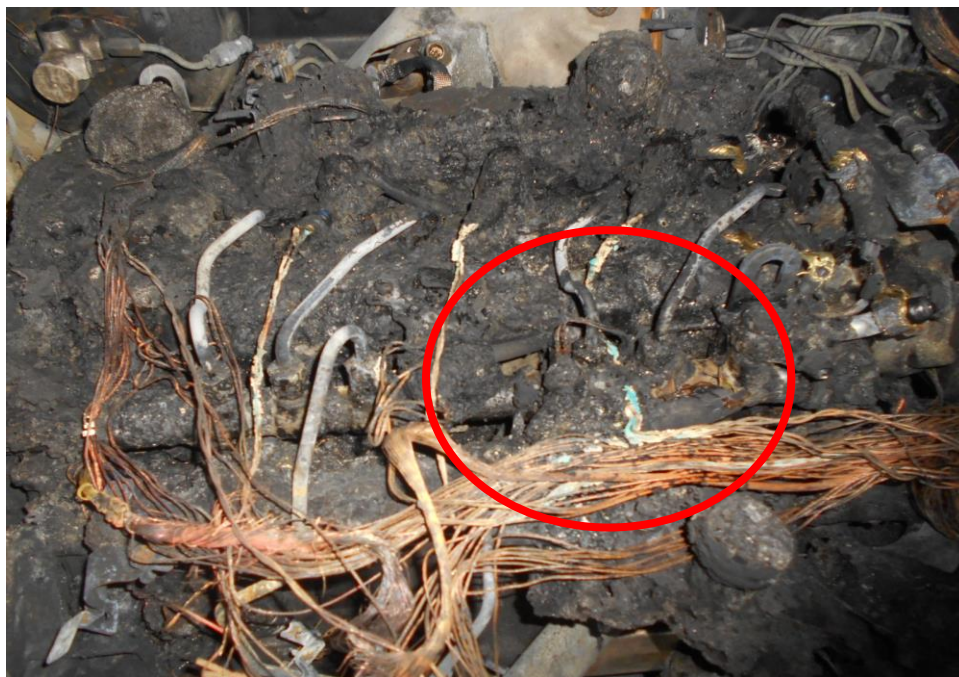
Photo 9 shows a closer view of the wirings with greenish residue found around the front centre portion of the engine compartment of the Insured Vehicle (red arrows). The presence of such greenish residue suggests occurrence of an electrical short circuit.
