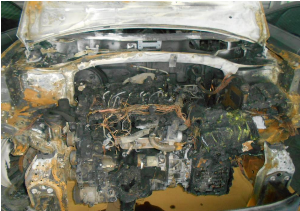
Photo 6 shows a general view of the engine compartment of the Insured Vehicle at the time of our inspection. Most of the components inside the engine compartment were found to be severely burnt and/or melted as a result of the fire.
