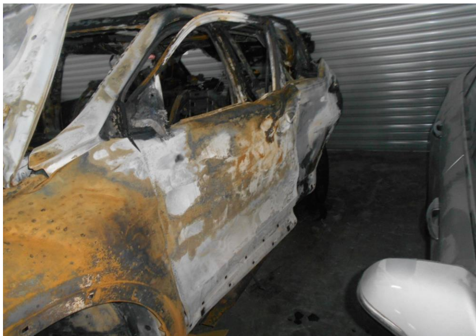
Photo 4 shows the general view of the left body of the Insured Vehicle at the time of our inspection. The Insured Vehicle was observed to have sustained extensive fire damage all around. Rust had accumulated all over the Insured Vehicle as a result of exposure to environmental condition for a period of time.
