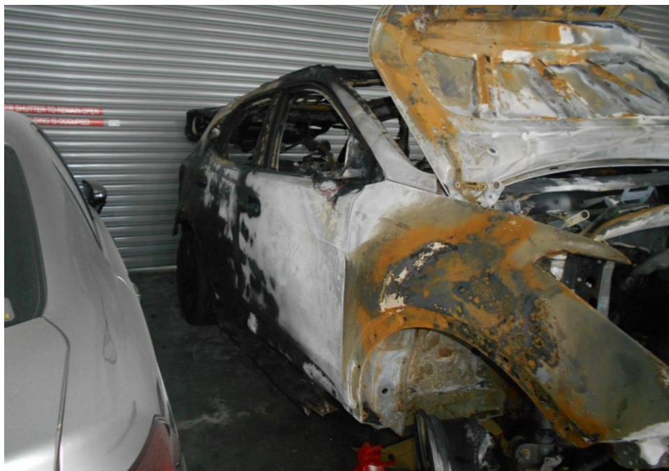
Photo 3 shows the general view of the right body of the Insured Vehicle at the time of our inspection. The Insured Vehicle was observed to have sustained extensive fire damage all around. Its engine compartment and interior compartment were completely burnt. Rust had accumulated all over the Insured Vehicle as a result of exposure to environmental condition for a period of time.
