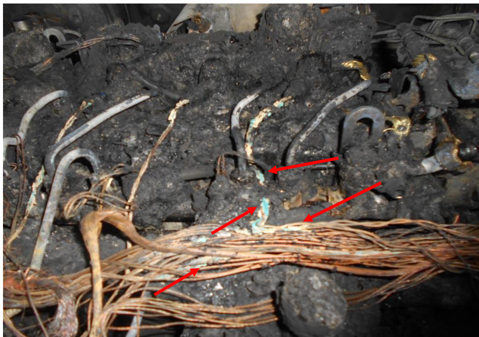
Photo 10 shows a close up view of the wirings with greenish residue found around the front centre portion of the engine compartment of the Insured Vehicle (red arrow). The presence of such greenish residue suggests occurrence of an electrical short circuit.
