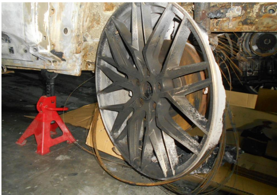
Photo 7 shows the non-standard rim found to be fitted on the Insured Vehicle at the time of our inspection. The 20- inch alloy rims fitted on the Insured Vehicle were not the standard type for the Insured Vehicle.
